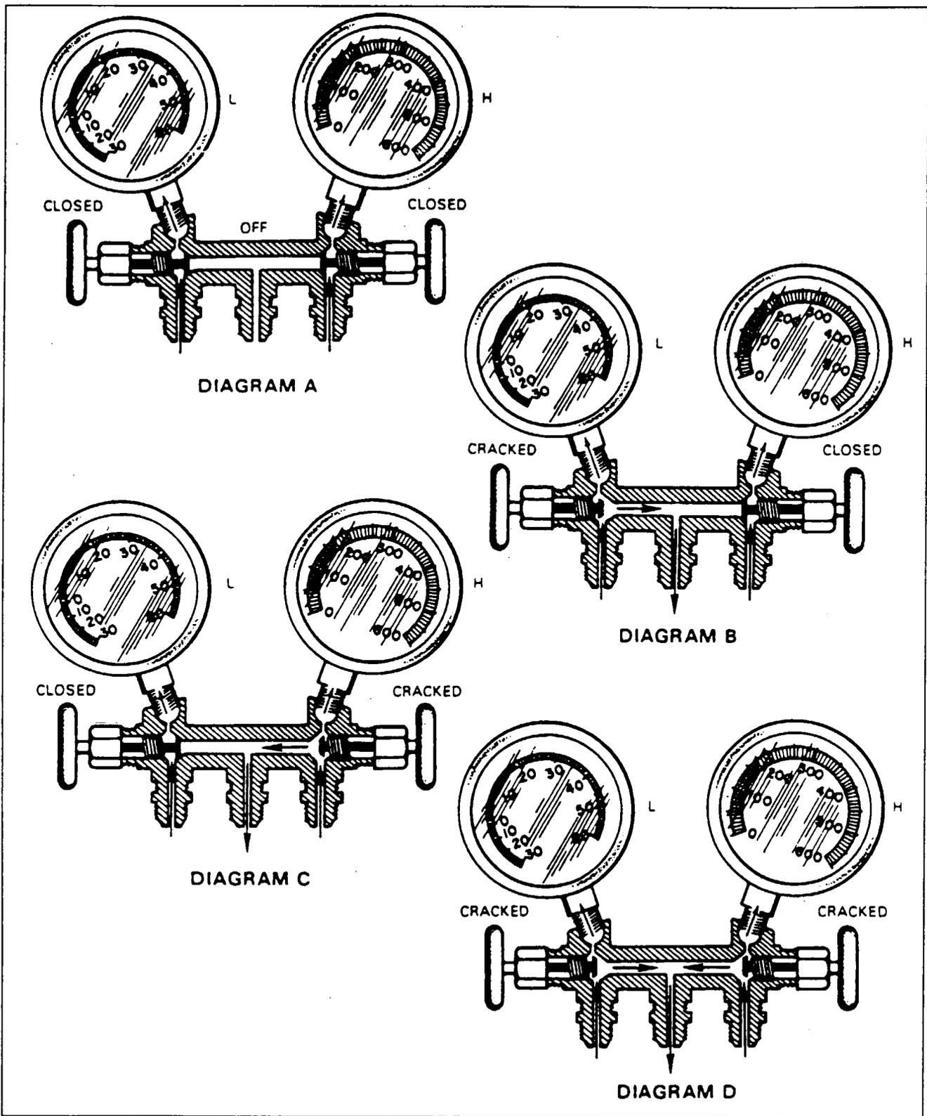
Figure 21-22. Manifold Set Operation
