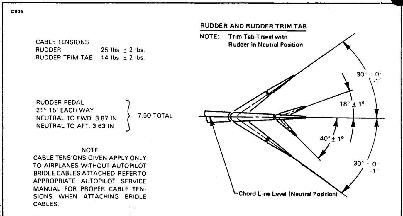
Figure 27-14. Rudder and Trim Tab Control Travels and Cable Tensions
