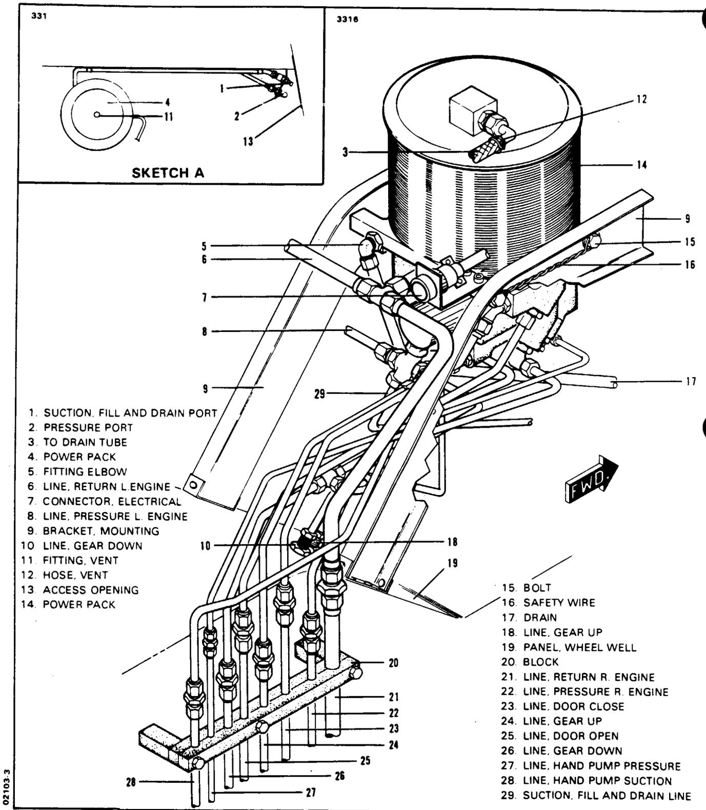
Figure 29-4. Power Pack Installation (Typical)
