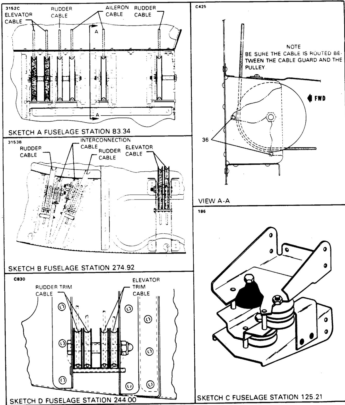
Figure 27-18. Elevator and Elevator Trim Controls (cont.)
