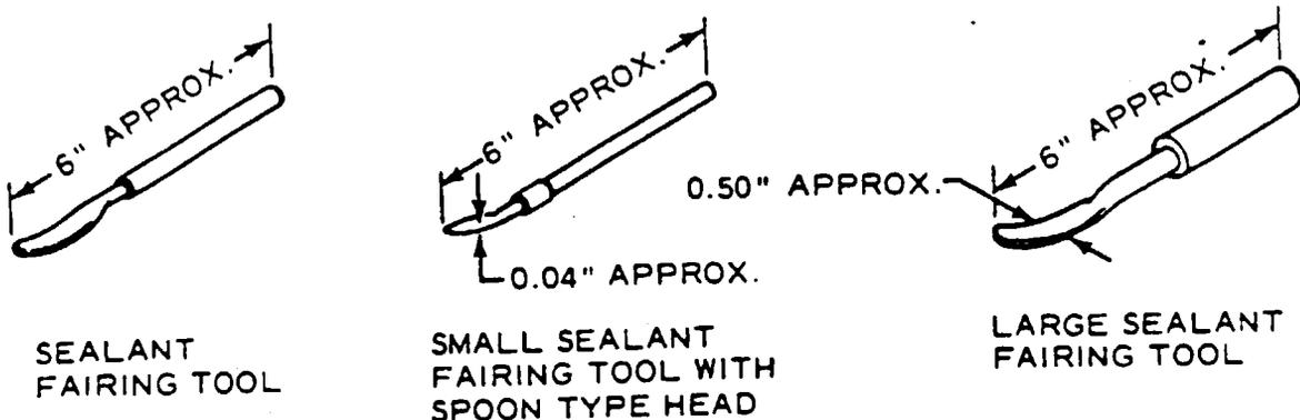
NOTE: THESE TOOLS MAY BE MADE OF 1/4 INCH DIAMETER BRONZE OR STEEL WELDING ROD AND MAY BE PLATED TO IMPROVE SMOOTHNESS.
