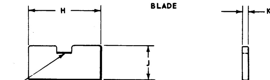
A WEAR NOTCH EXCEEDING .010 IN DEPTH IN THIS AREA INDICATES THAT BLADE SHOULD BE DISCARDED.
