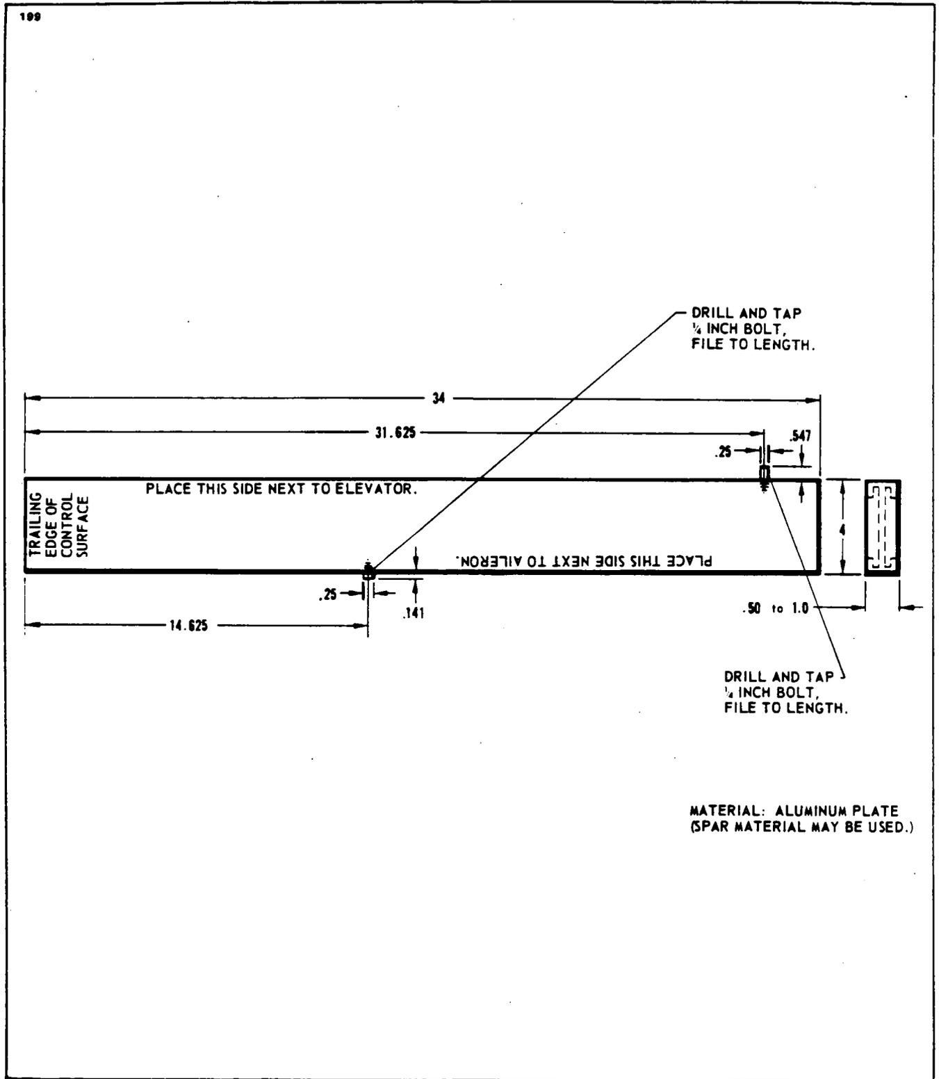
Figure 95-4. Fabricated Aileron and Elevator Rigging Tool
