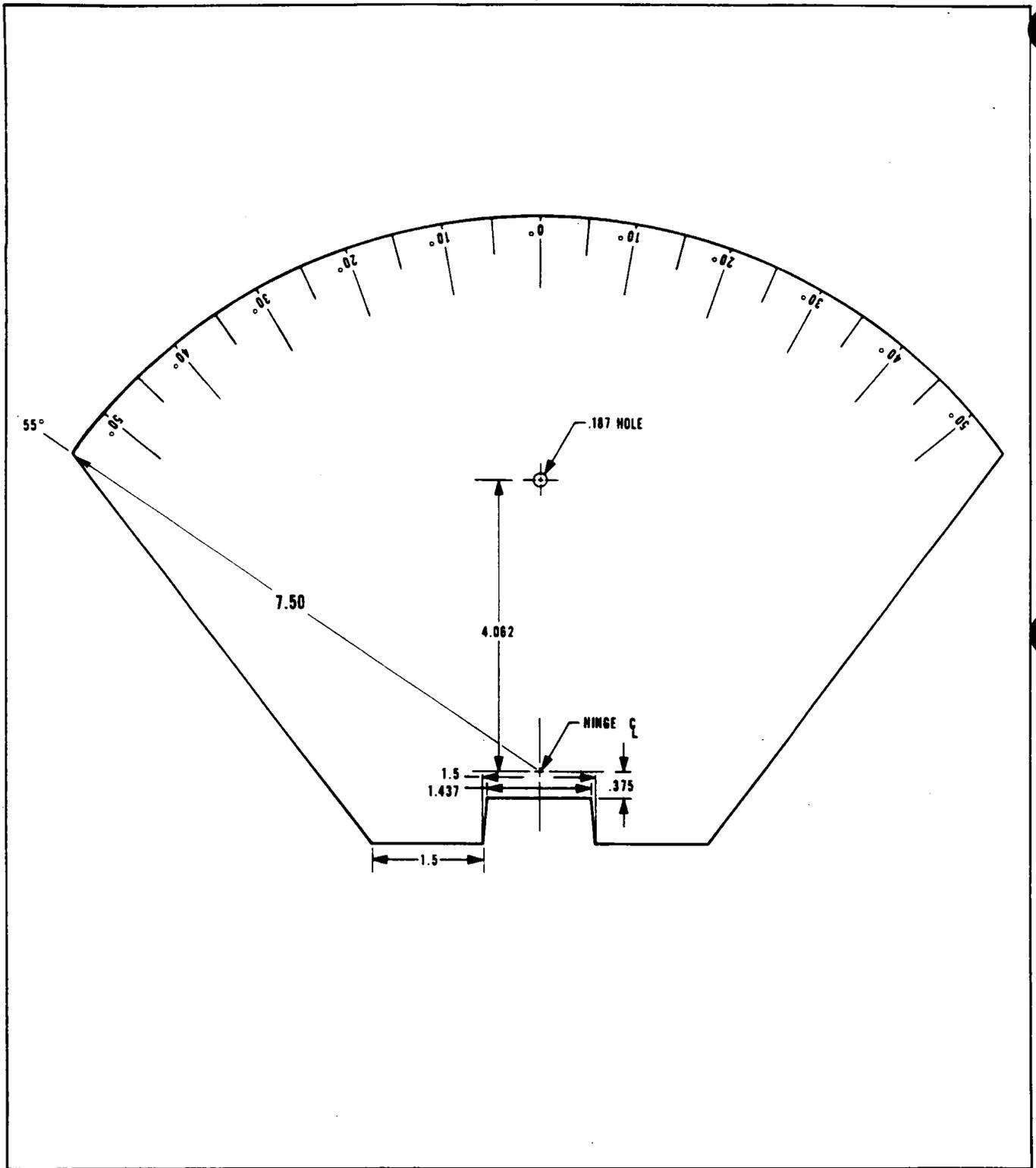
Figure 95-6. Fabricated Rudder Trim Tab Rigging Tool
