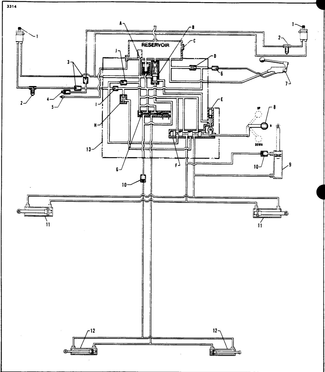
Figure 29-1. Schematic Diagram of Hydraulic System
