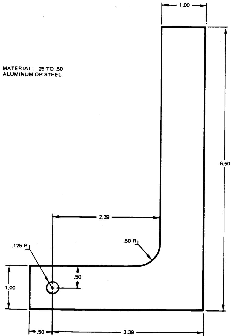
Figure 95-3. Fabricated Bellcrank Rigging Tool
