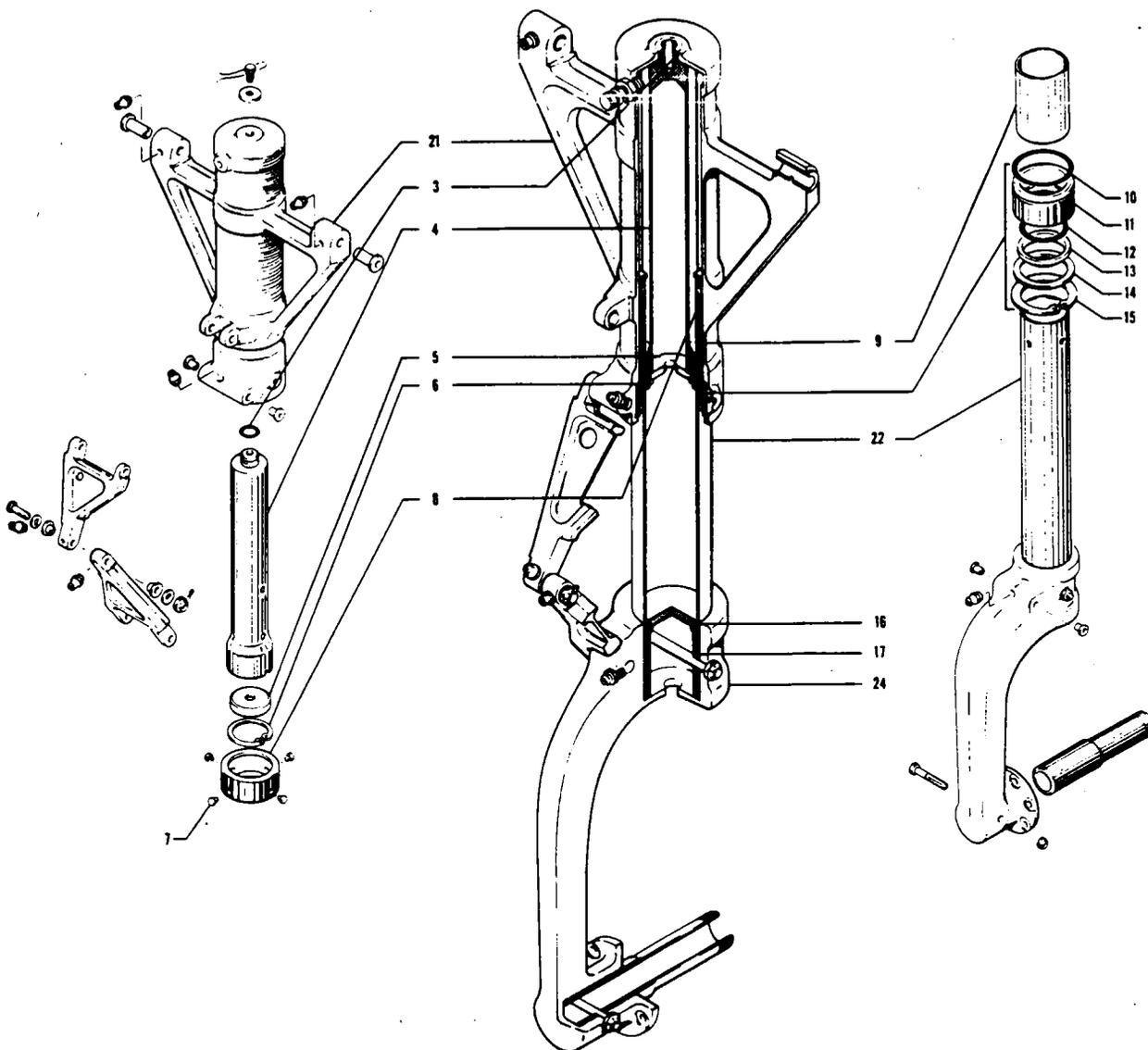
Figure 32-2. Main Gear Oleo Strut Assembly (cont.)
