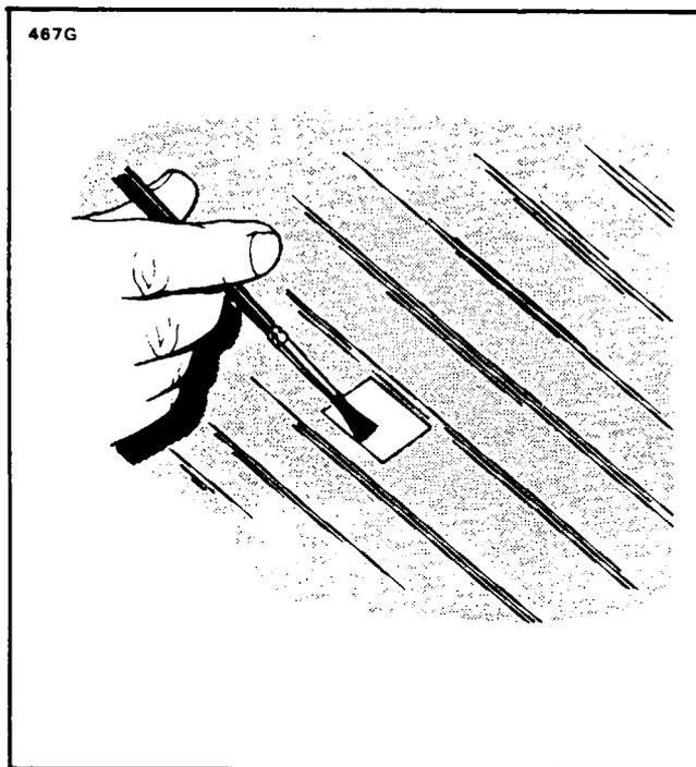
Figure 30-9. Cementing Buffed Area and Patch
