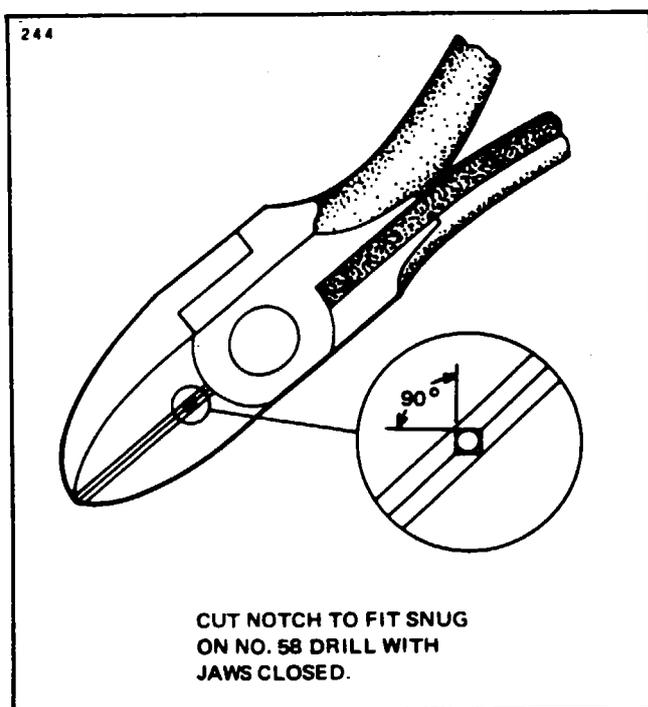
Figure 95-20. Modified Pliers for Ignition Harness
