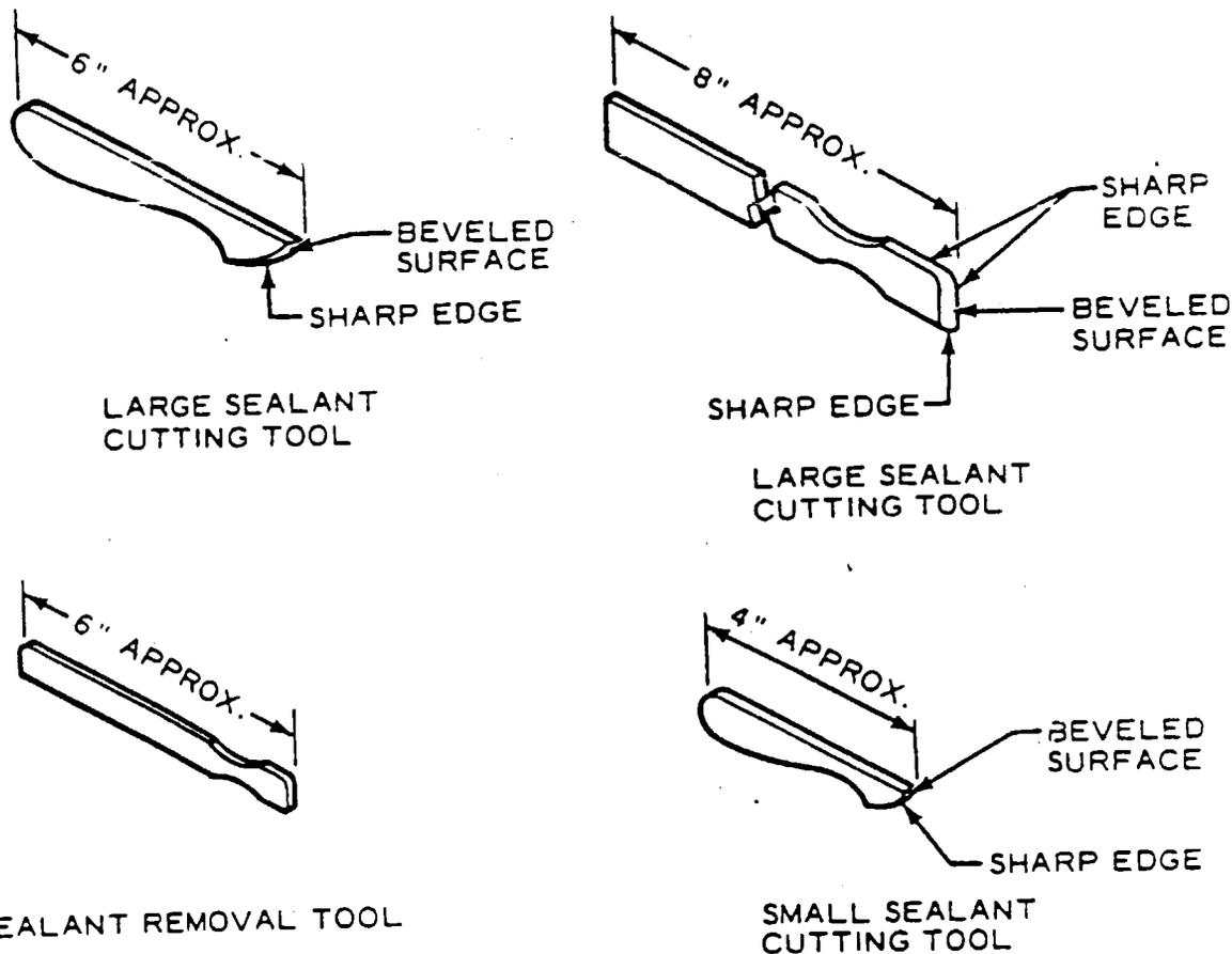
NOTE: THE ABOVE TOOLS SHOULD BE MADE OF HARDWOOD TO REDUCE THE POSSIBILITY OF STRUCTURAL DAMAGE.
