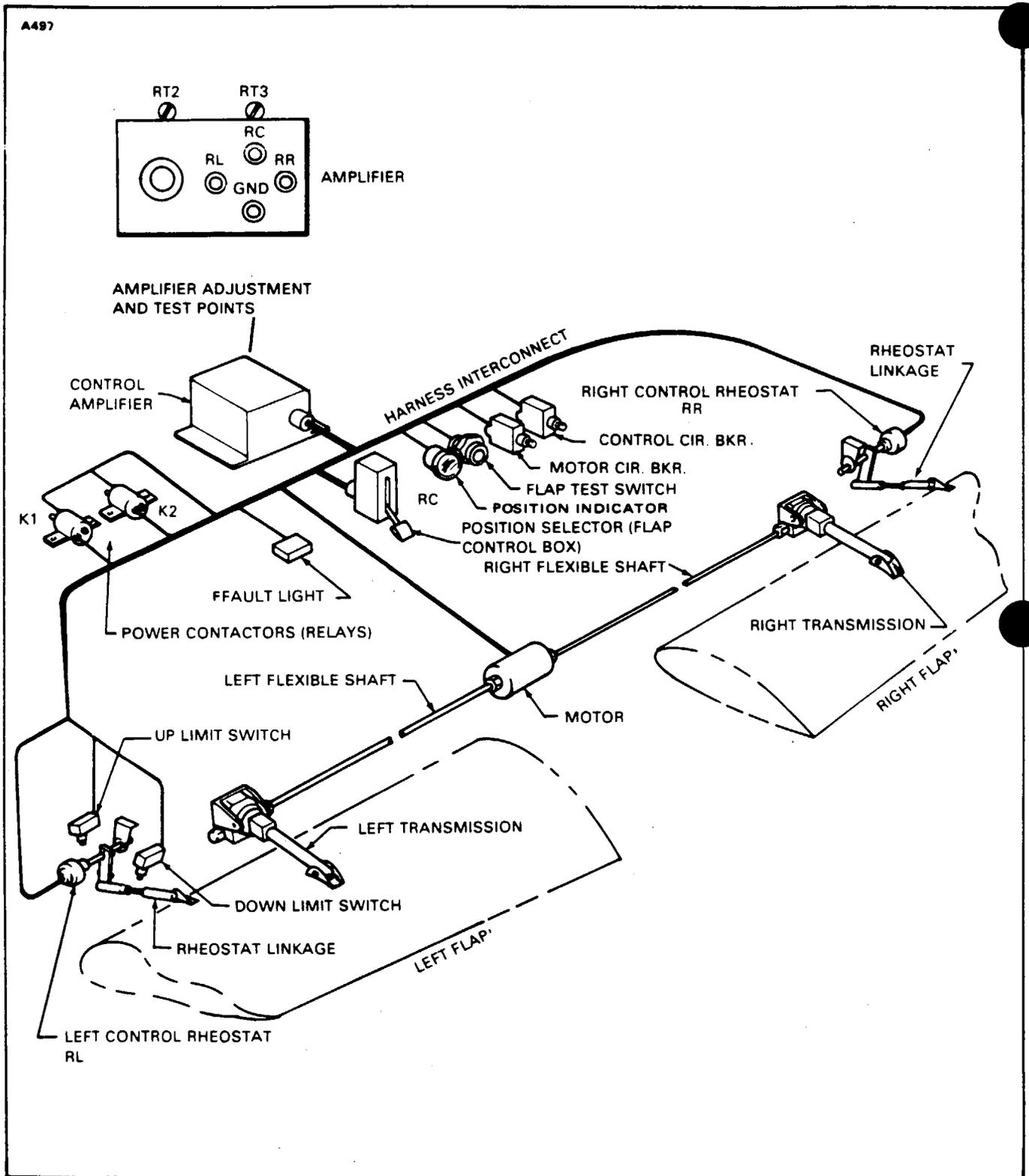
Figure 27-25. Flap System Diagram
