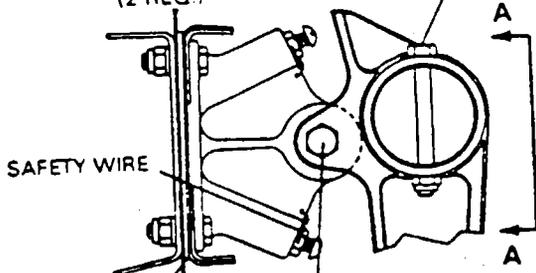
SHIM AS REQUIRED BETWEEN DOUBLER AND FRONT FACE OF REAR SPAR. IT IS NOT PERMISSIBLE TO SHIM MORE THAN .091 THICKNESS. OR TO USE ANY COMBINATION OF SHIMS. REFER TO PARTS CATALOG FOR PROPER SHIM PART NUMBER.
