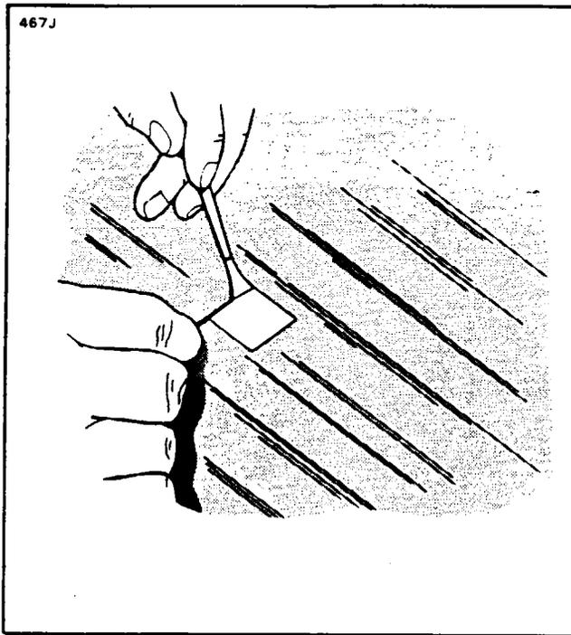
Figure 30-11. Placing and Stitching Gum
