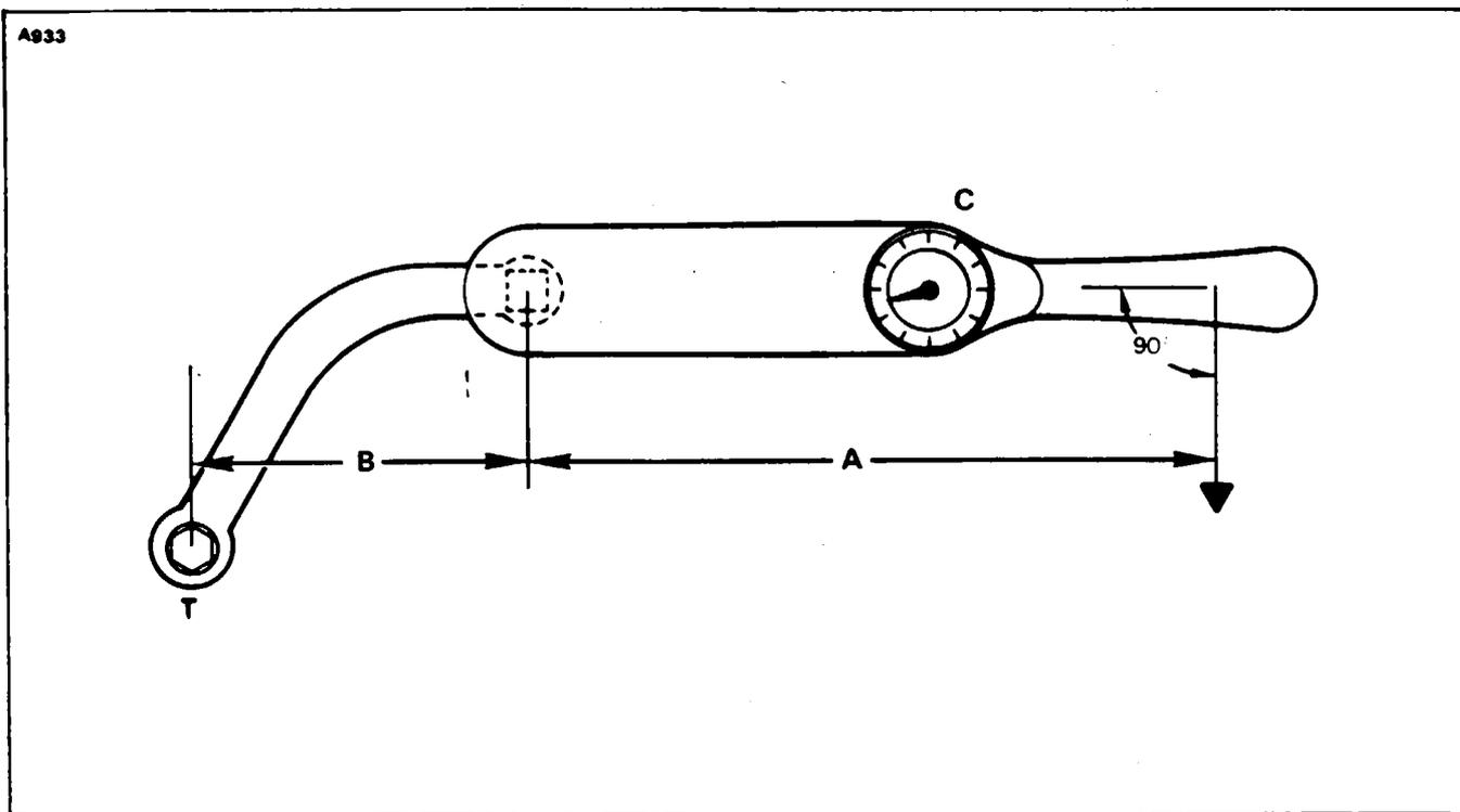
Figure 95-17. Torque Wrench Extension
