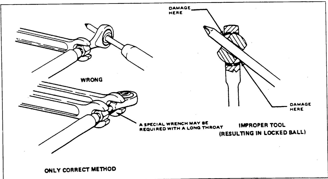
Figure 20-2. Method of Installing Rod End Bearings
