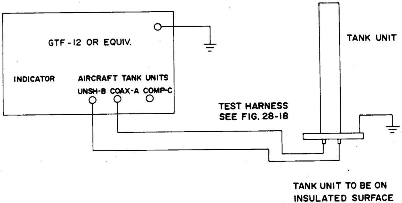
Figure 28-17. Tank Unit Test Set-Up
