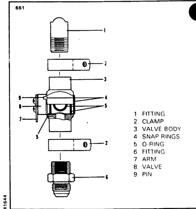
Figure 28-10. Fuel Shutoff Valve
