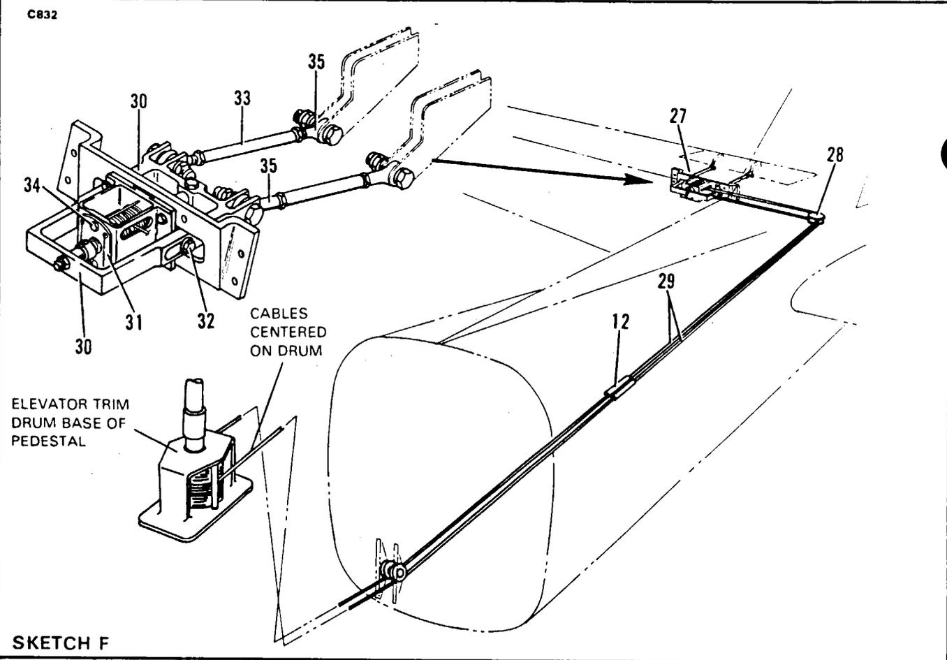
Figure 27-18. Elevator and Elevator Trim Controls (cont.)
