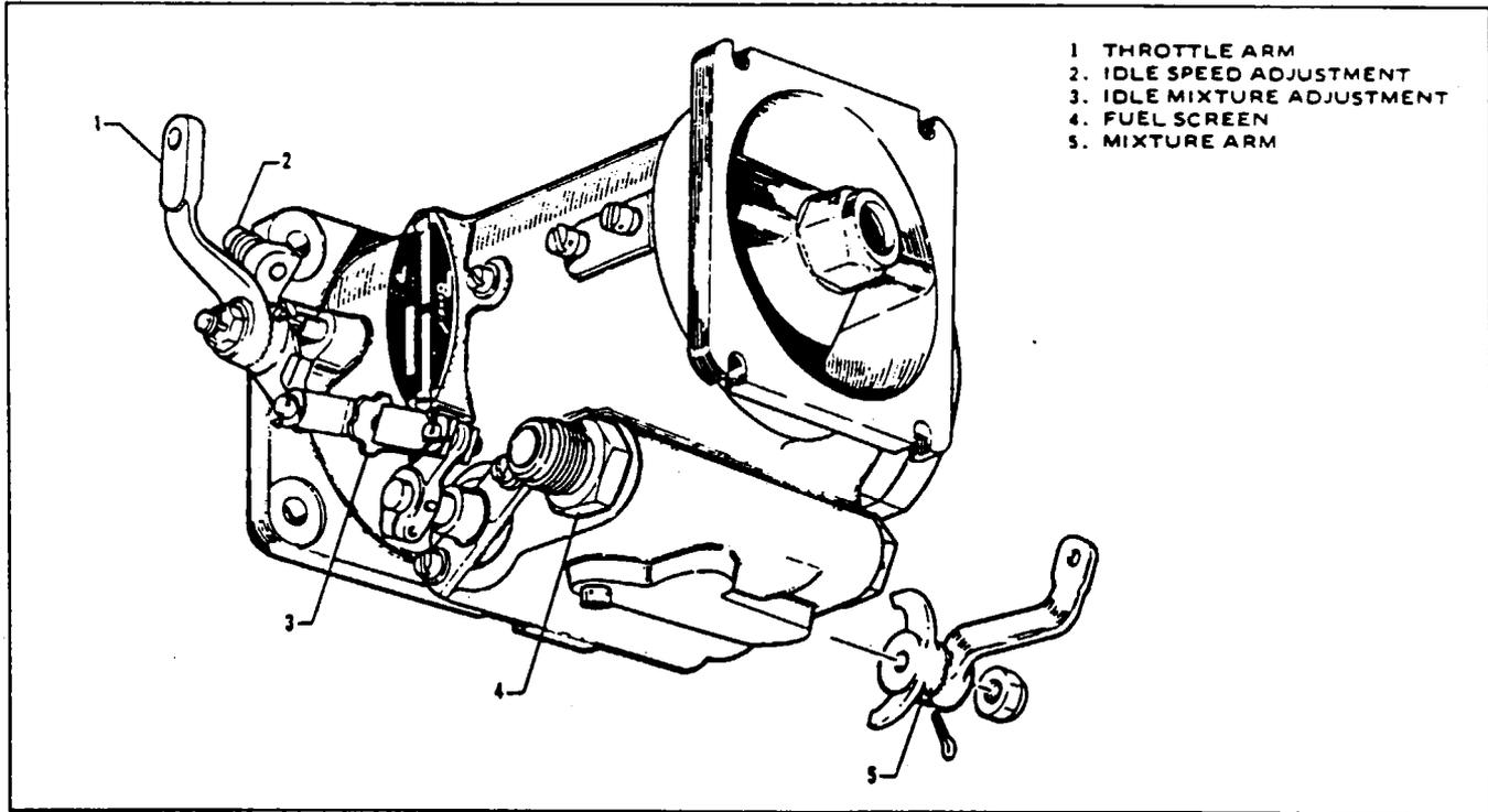
Figure 73-1. Fuel Injector
