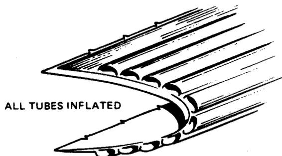
Figure 30-2. Pneumatic Deicer Boots Operation (Typical)
