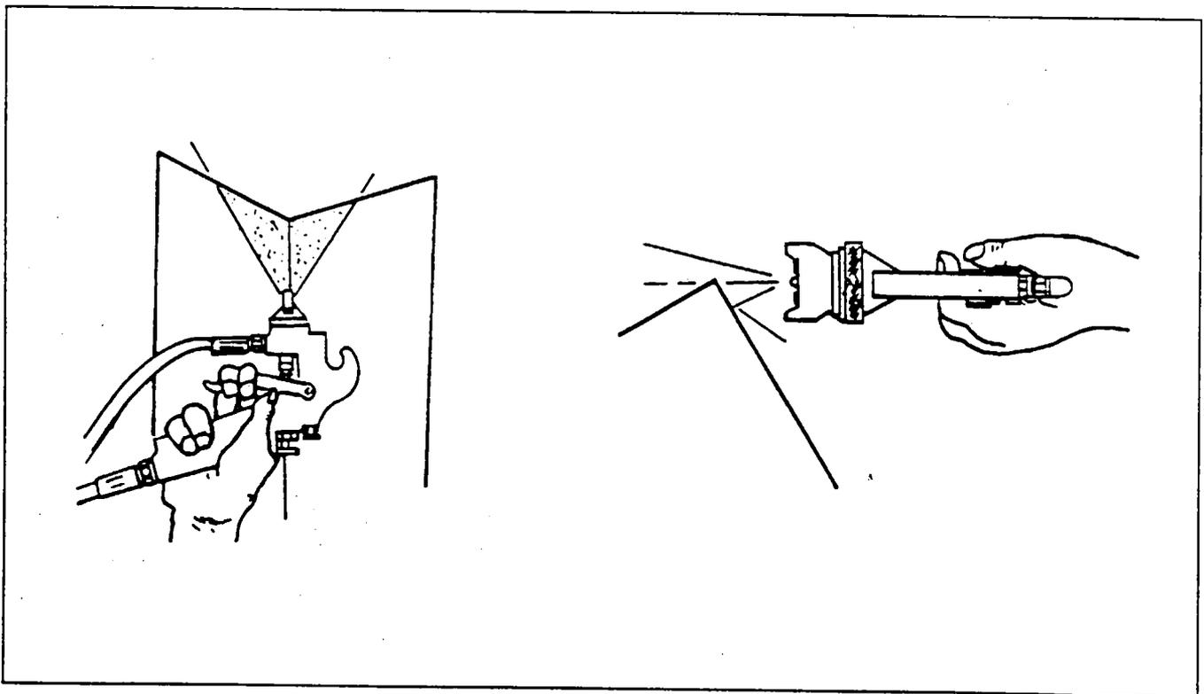
Figure 20-9. Spraying Corners
