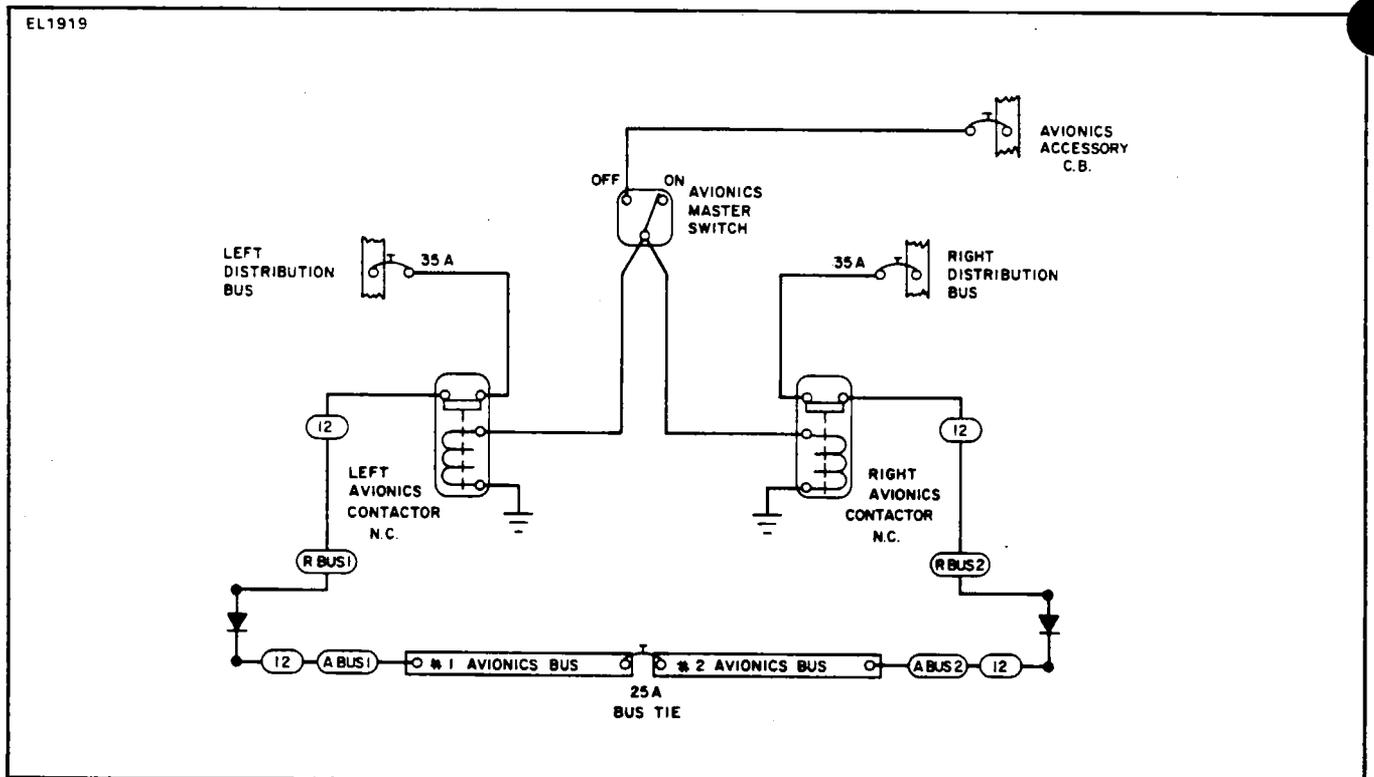
Figure 23-4. Avionics Master and Emergency Switch Circuit
