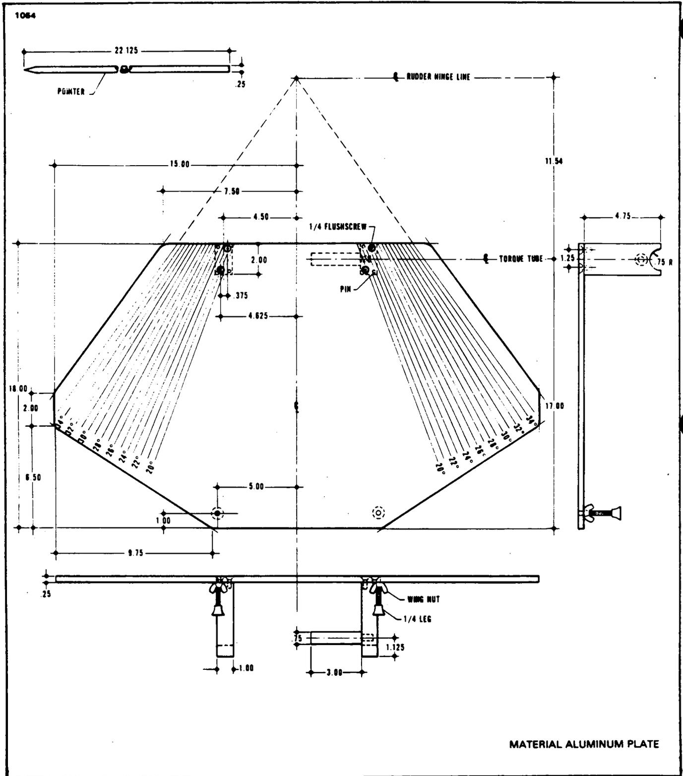
Figure 95-5. Fabricated Rudder Rigging Tool
