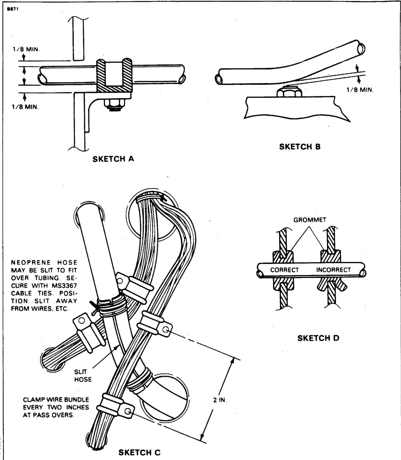
Figure 35-3. Oxygen Tubing Installations
