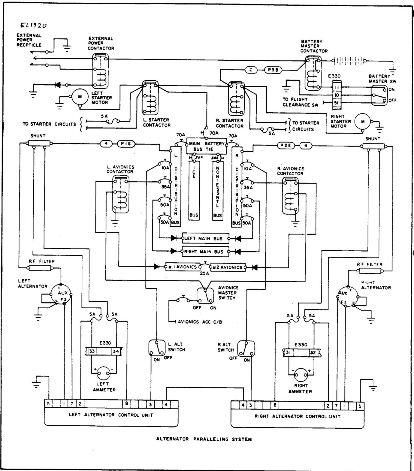
Figure 24-2. Electrical Power Distribution System
