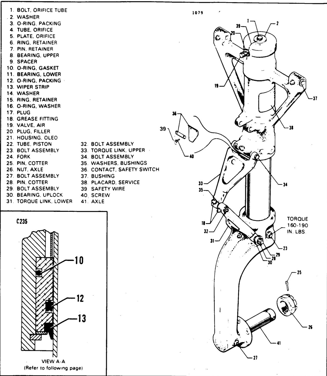
Figure 32-2. Main Gear Oleo Strut Assembly
