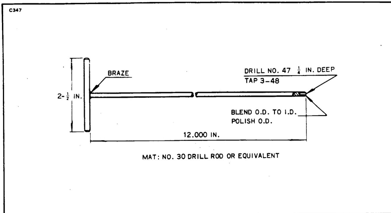
Figure 95-19. Assembly Tool - Ignition Harness Insulating Sleeves
