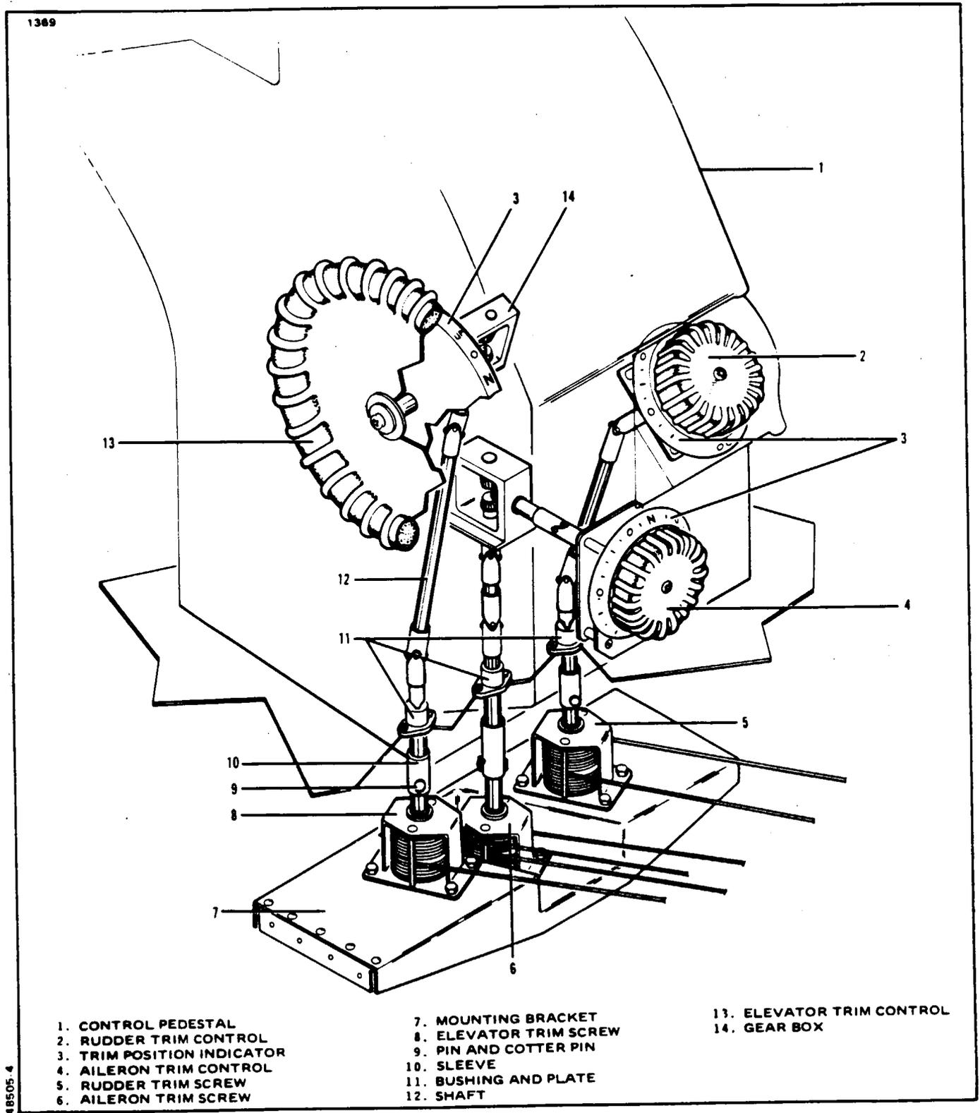
Figure 27-10. Trim Controls Installation
