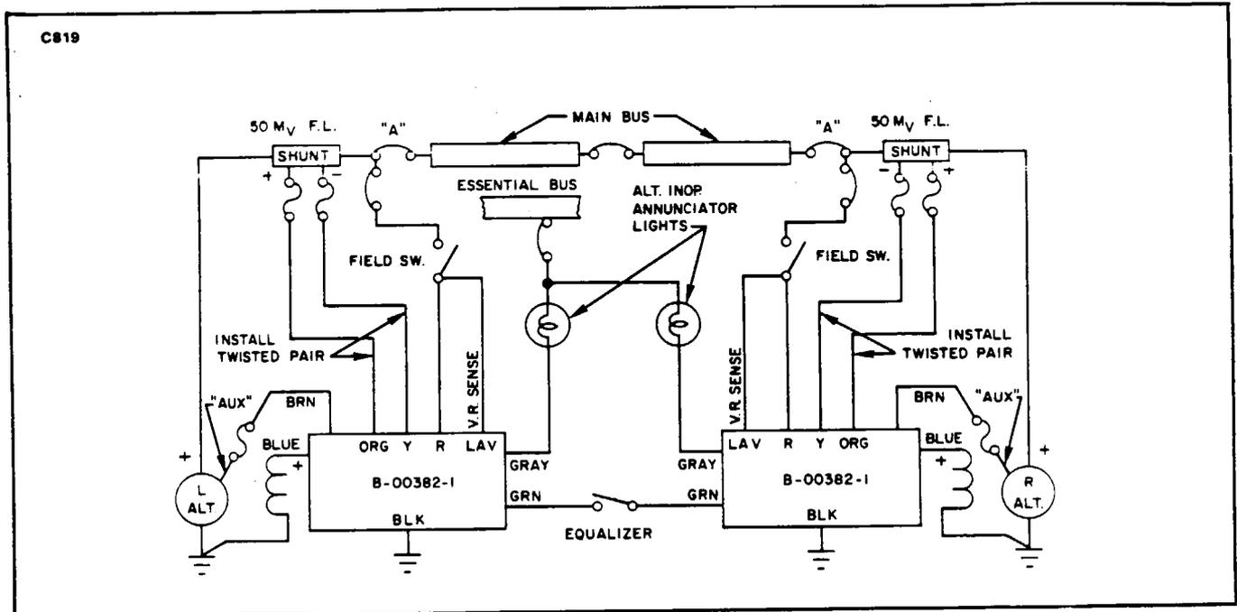
Figure 24-3. Lamar Model B-00382-1, Typical System Application
