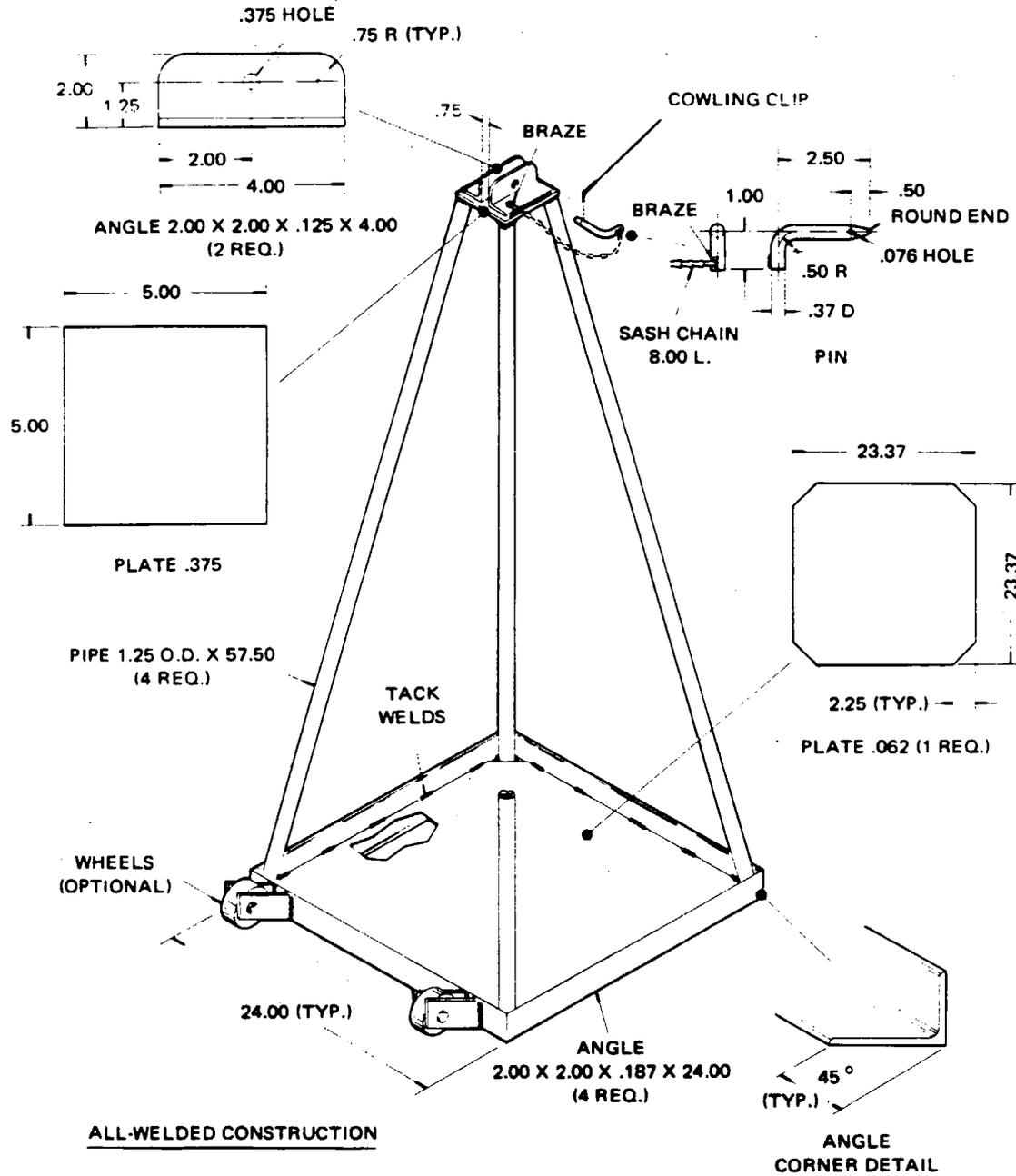
Figure 95-2. Fabricated Tail Stand
