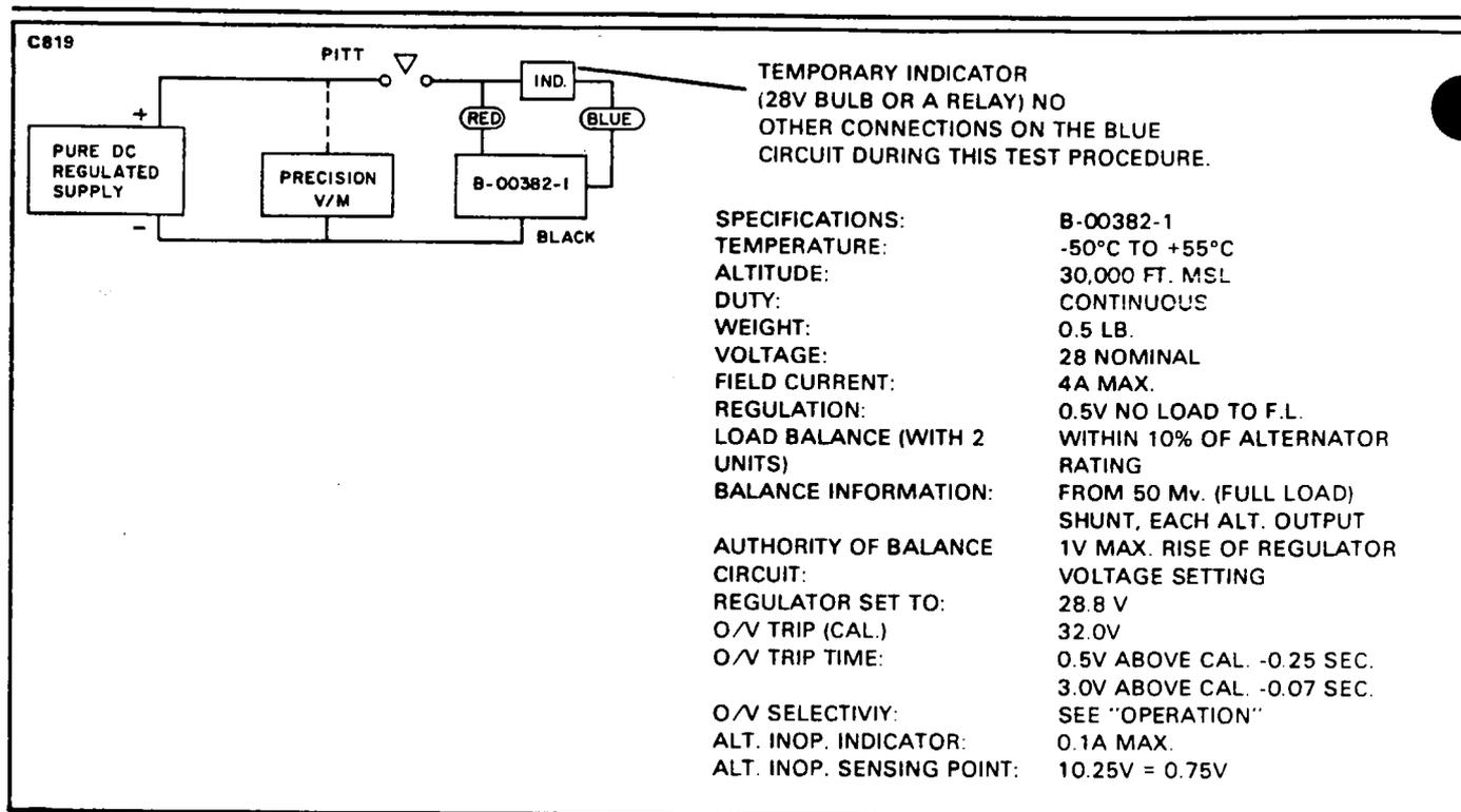
Figure 24-4. Lamar B-00382-1 A.C.U. Test Specifications
