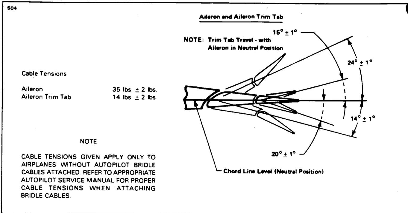
Figure 27-11. Aileron Control Travels and Cable Tension
