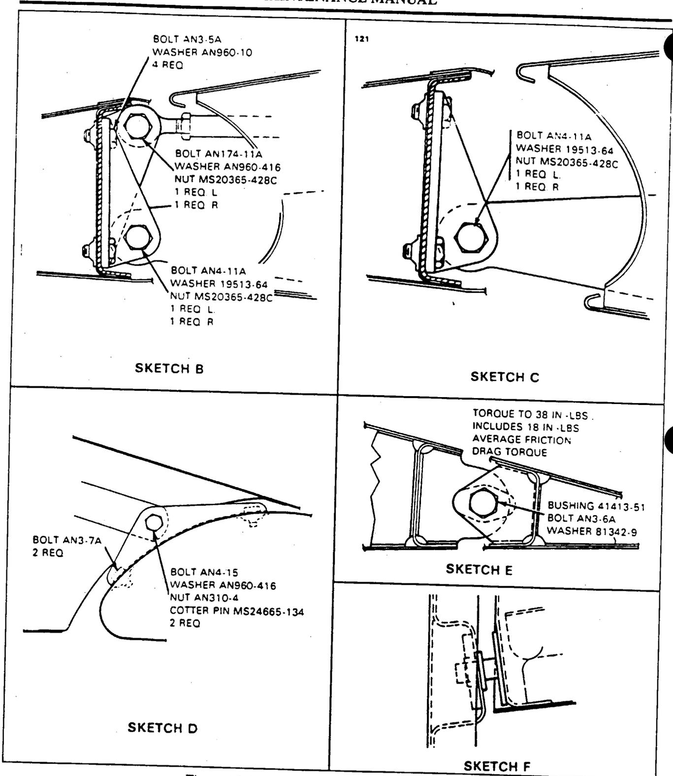
Figure 57-5. Aileron and Flap Installation (cont.)
