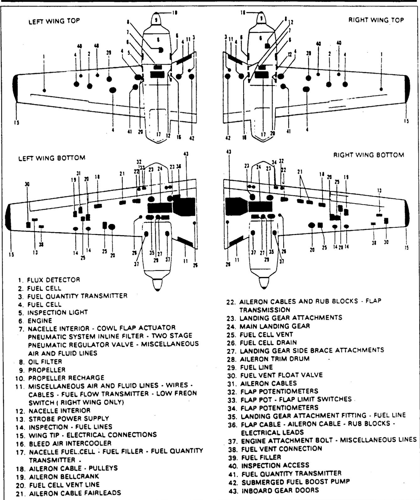
Figure 6-3 Access Plates and Panels (cont. )
