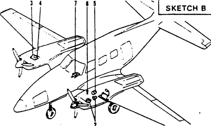
Figure 12-6. Lubrication Chart (Power Plant, Propeller and Cowl Flap)
