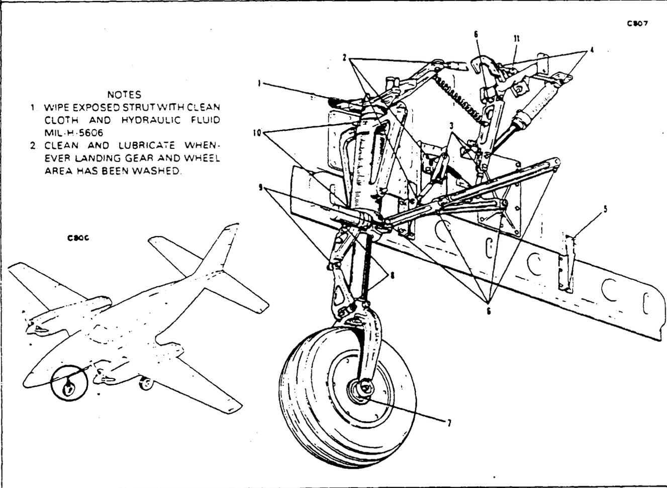
Figure 12-4. Lubrication Chart (Landing Gear, Nose)
