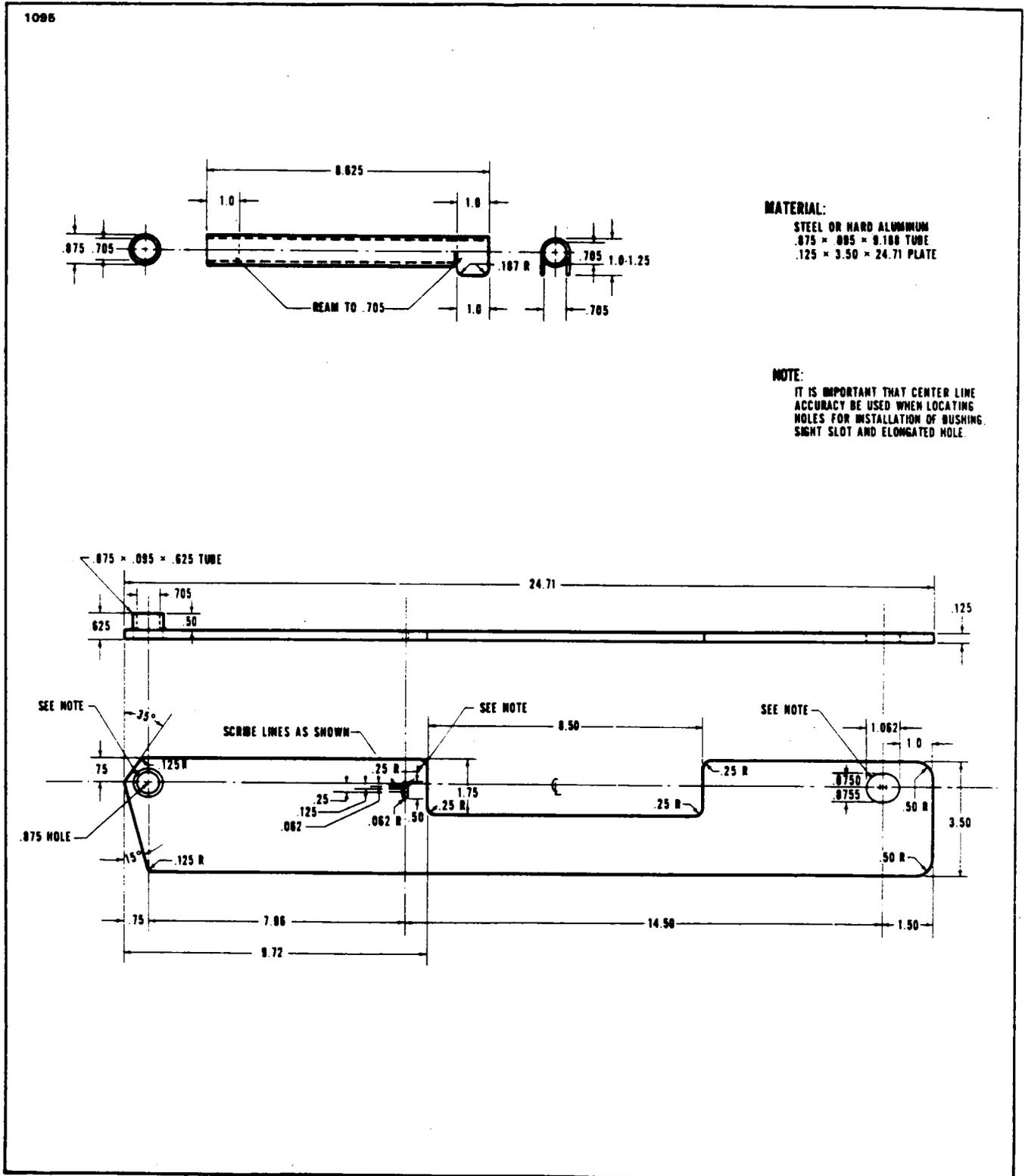
Figure 95-7. Fabricated Tool. Checking Nose Gear Link Travel
