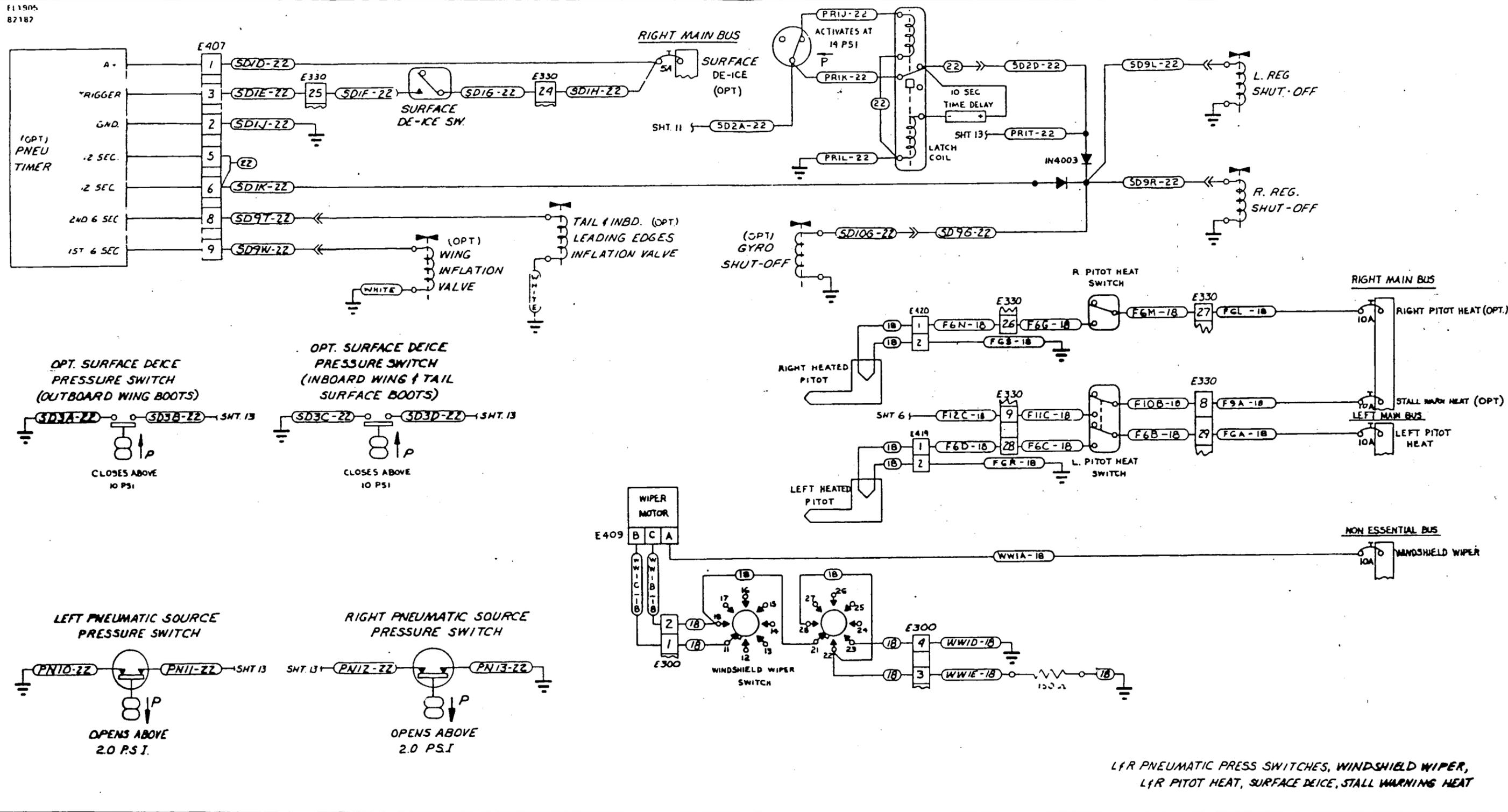
L/R PNEUMATIC PRESS SWITCHES, WINDSHIELD WIPER, L/R PITOT HEAT, SURFACE DEICE, STALL WARNING HEAT
