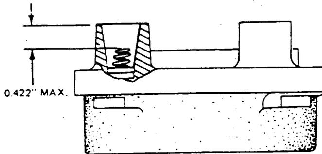
Figure 74-1. Height of Spring in Distributor block Tower
