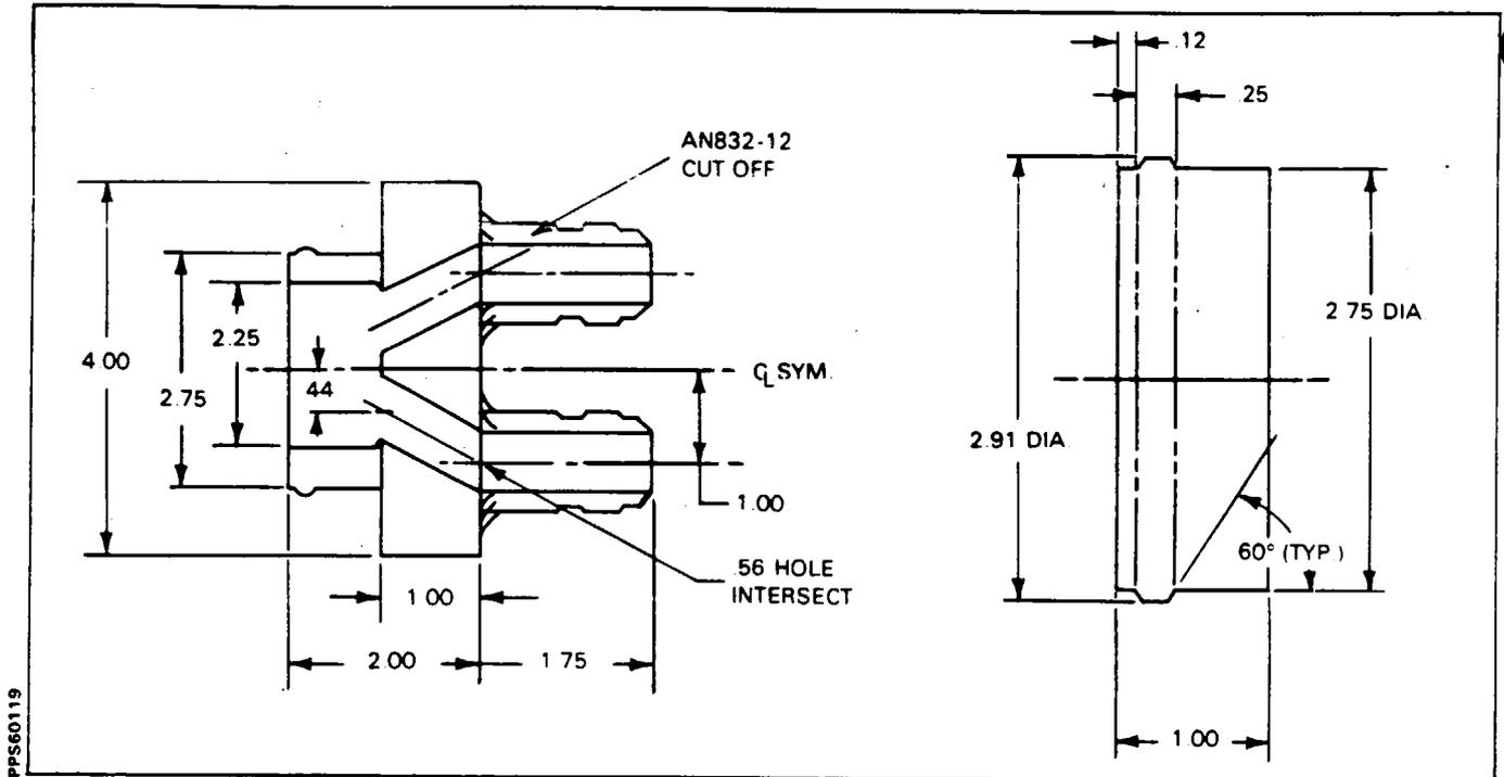
Figure 95-14. Fabricated Pressure Test Adapter
