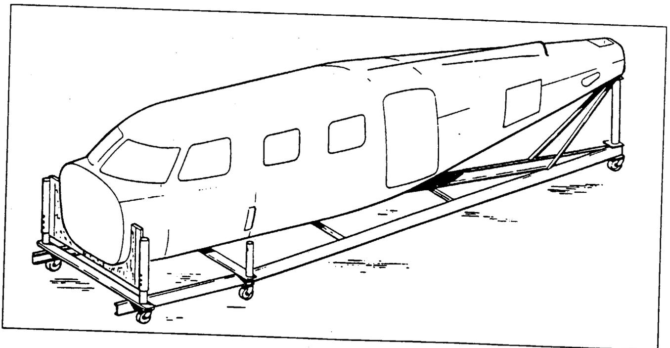
Figure 57-3. Fuselage Cradle (Typical)
