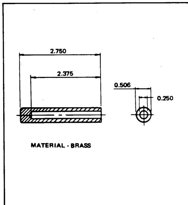
Figure 95-21. Ferrule Seating Tool-Ignition Harness
