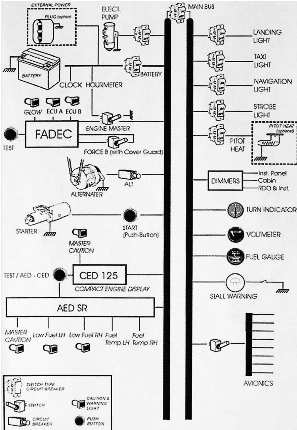
Figure 1-4a Basic Wiring of the Electrical System with Circuit Breaker Alternator
