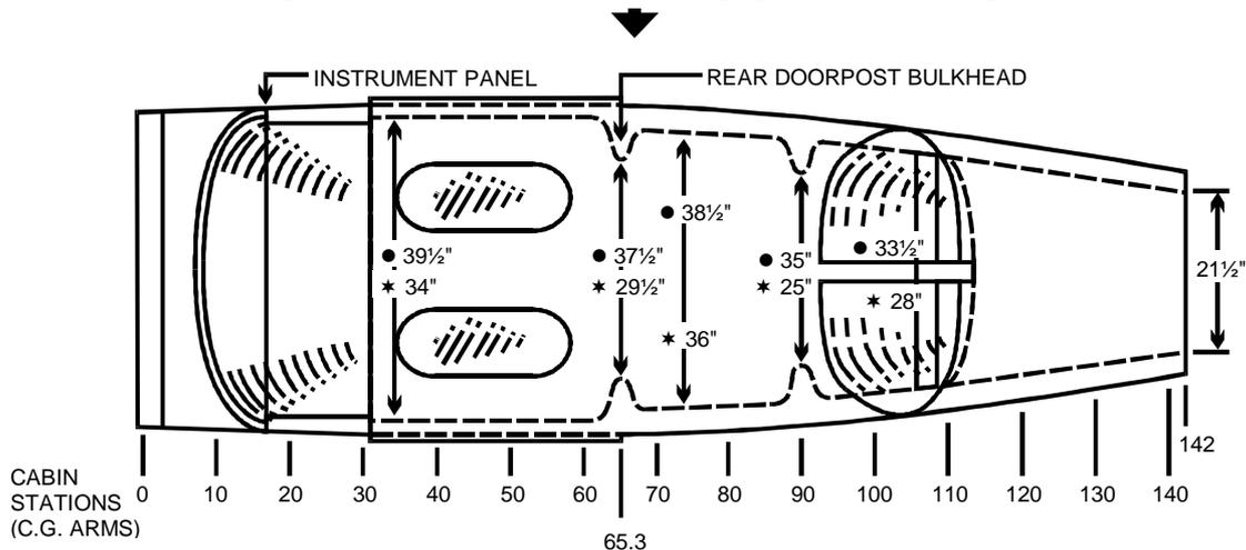
Figure 6-4. Internal Cabin Dimensions
