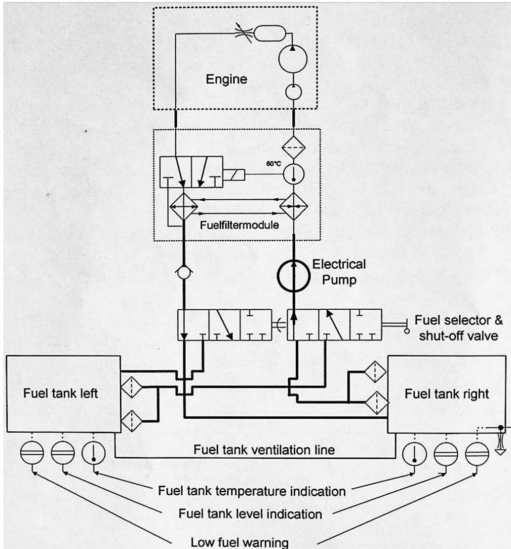
Figure 1-3a Scheme of the Fuel System (Left, Right)
