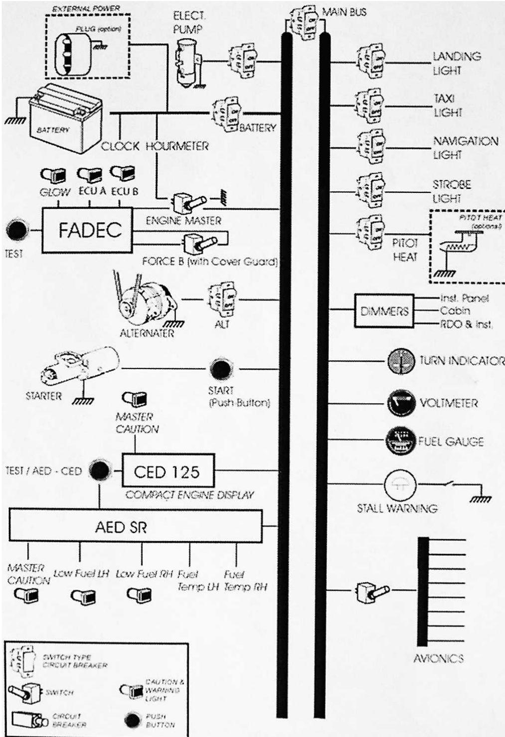
Figure 1-4b Basic Wiring of the Electrical System with Switch Alternator
