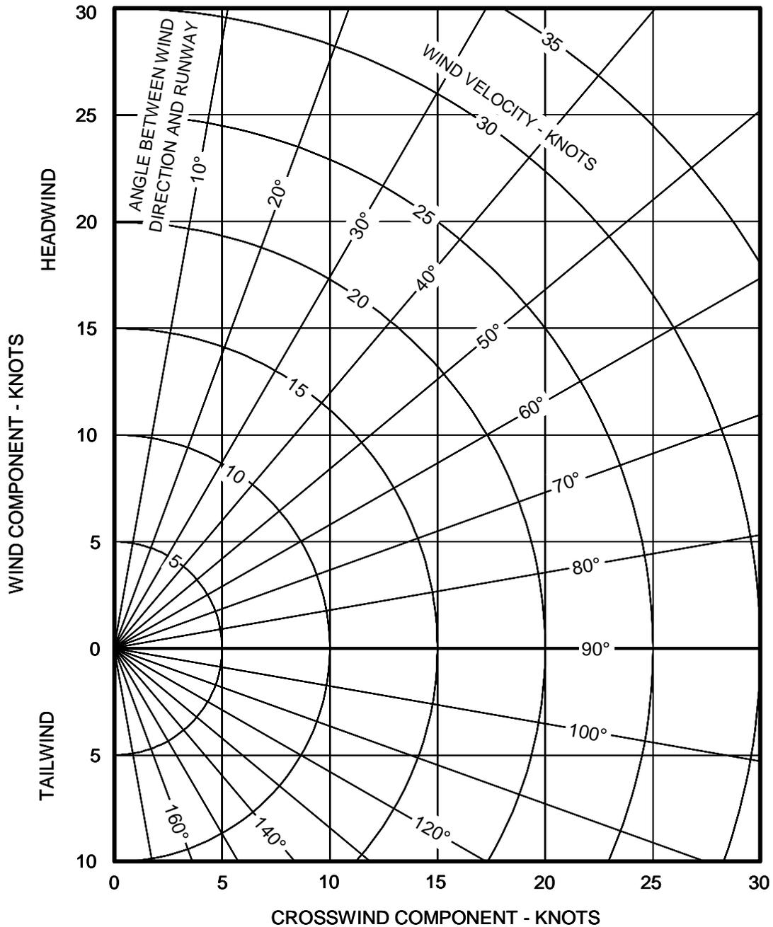
Figure 5-4. Wind Components
