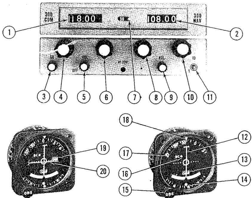
1. RECEIVER-TRANSMITTER FREQUENCY INDICATOR.
