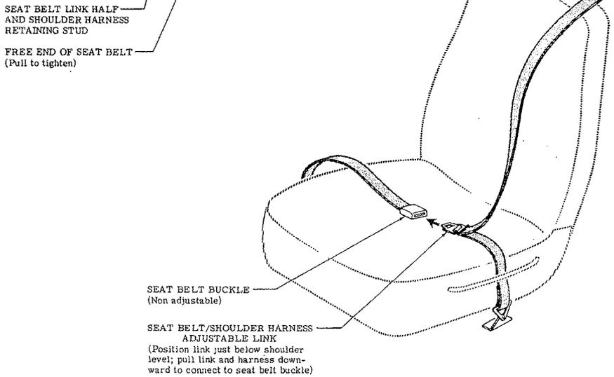
Figure 7-4. Seat Belts and Shoulder Harnesses
