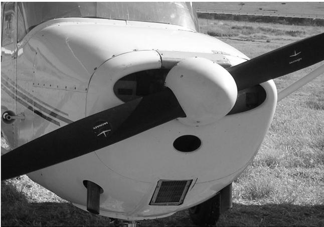
Check condition and security of air filter. Air filter should be clear of any dust or other foreign matter. Visually check exhaust for signs of wear, if engine is cool check exhaust is secure. Check landing light and taxi lights for condition and security (if cowl mounted).
