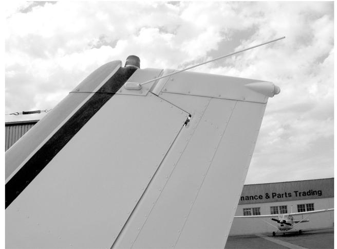
Check beacon, aerials and rear navigation light undamaged and secure.
