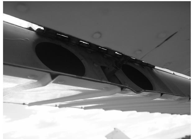
Check for damage to surface and security of all hinges, control connections, and flutter weights.
