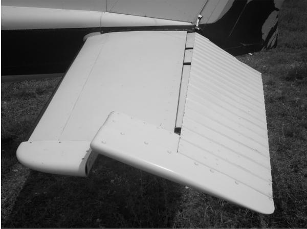
Check top, bottom, and side surfaces for any damage, ensure balance weights and fairings secure.
