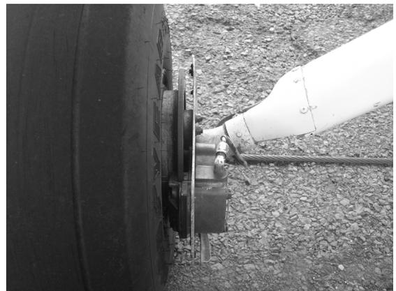
Check the security and condition of hydraulic lines, disc brake assembly and all fastenings.
