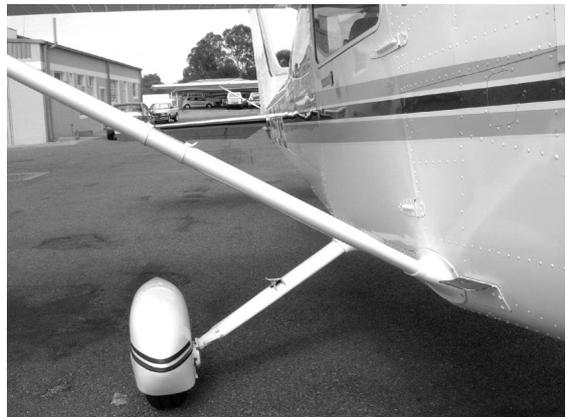
Check the condition and security of fairing (if fitted), strut and wheel.
