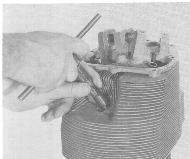
FIGURE 5-5. EXPANDING SPARK PLUG HOLE HELICAL INSERT.
