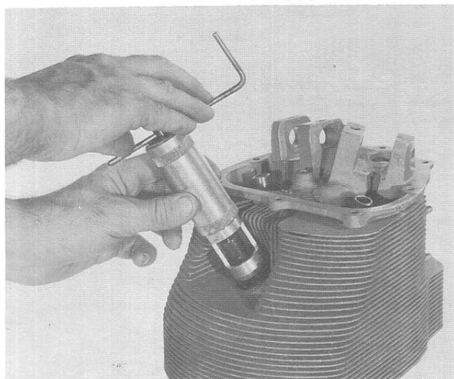
FIGURE 5-4. INSTALLING SPARK PLUG HOLE HELICAL INSERT.
