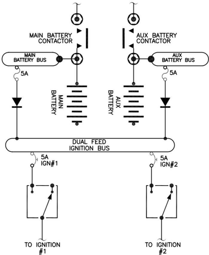
Figure 3. Ignition System Power
