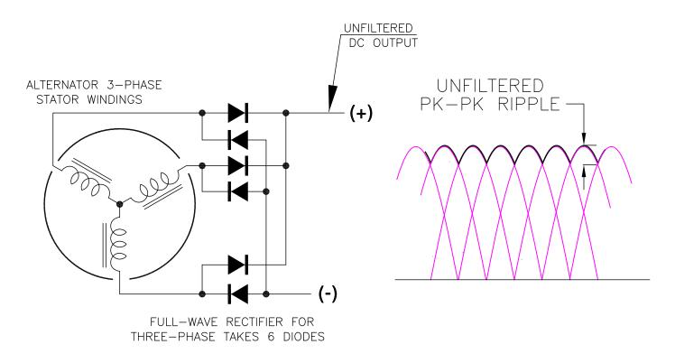
THREE PHASE AC OUTPUTS OVERLAP EACH OTHER BY 1/3 THEIR PERIODS. THE RESULTING FULL WAVE RECTIFICATION HAS A VERY LOW PK-PK RIPPLE AMPLITUDE WITHOUT FILTERING. COMPARE THIS WITH THE UNFILTERED OUTPUT IN FIGURE 16-1.
