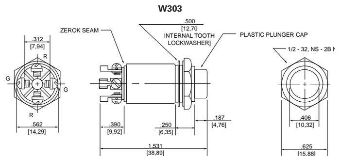
SUPPLIED WITH FOUR TERMINAL SCREWS, LOCK WASHERS AND LUGS.
