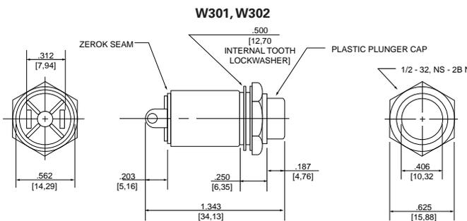
SUPPLIED WITH TWO TERMINAL SCREWS, LOCK WASHERS AND LUGS.
