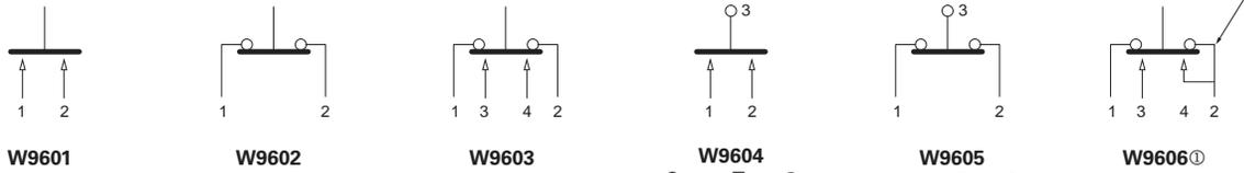
① For W9606 or SPDT circuit, mount terminal jumper to terminal #2 and #4.
