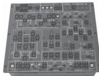
Sensing & Controls supplies advanced overhead panels to aircraft manufacturers who require high performance cockpit panels incorporating several hundred switches and indicators with ARINC 429 bus communication. Customers can also choose features such as logic and power supply redundancy, as well as LED lighting for both panel and indication. This integration of lighting, circuitry, and components leads to improved system reliability and low MTBF/MTBR.
