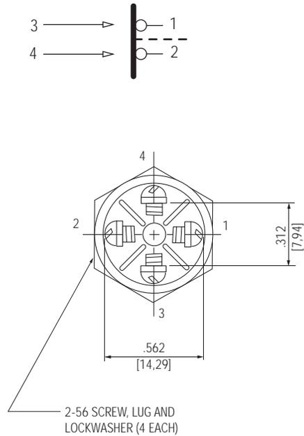
Mounting and terminal hardware supplied unassembled.
