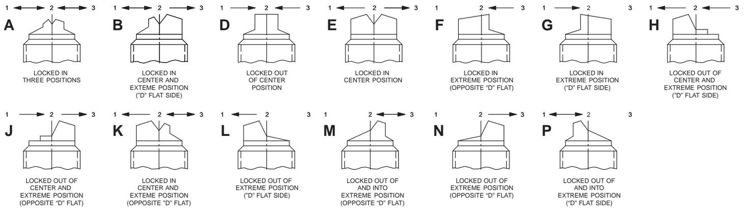
Notes: 1. Arrows (<>>) indicated lever must be unlocked to move against the arrow direction.
