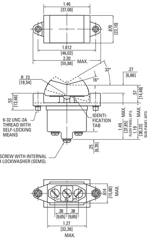
\*6-32 TERMINAL SCREW WITH INTERNAL TOOTH LOCKWASHER (SEMS).
