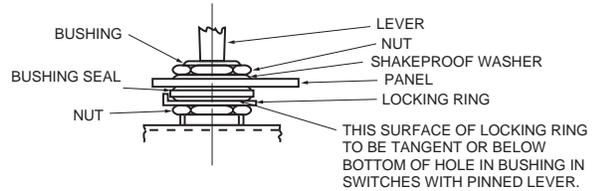
BUSHING SEAL TO BE ASSEMBLED SO THAT SURFACE, WITH MARKING "BOTTOM," IS DOWN. LOCKING RING CAN BE ASSEMBLED WITH EAR EITHER UP OR DOWN.
