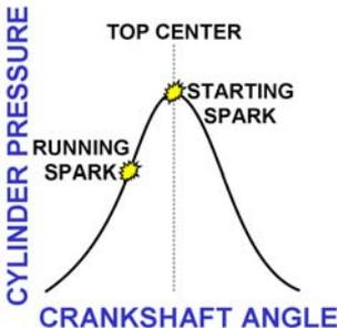
Ignition timing must be advanced to get maximum power output from a combustion engine at high RPM. If we try to start the engine with advanced ignition timing, combustion occurs too early and the engine kicks back and fails to start. Starting ignition can be improved by retarding (delaying) ignition timing until the piston is close to the top of the
