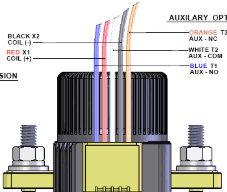
WIRE SPEC: SILICONE, 22AWG, -40C-150C, UL: VW-1
