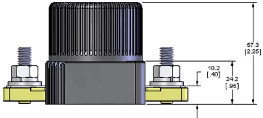
The polarity of the power terminals was previously shown reverse from what is correct and what is now indicated. The polarity is important only for switching the "Maximum Break, 2 cycles" when the voltage is over 100 Vdc.
