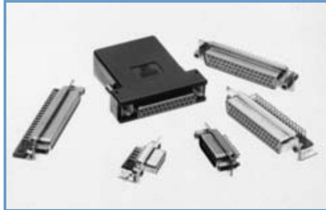
Harmo-D Series connectors are Military/Industrial quality rectangular connectors designed for use in sheltered, mildly corrosive environments having a wide range of temperature, pressure and humidity changes. These fixed contact connectors are qualified to MIL-DTL-24308 and meet the performance requirements of IEC 807-2, Performance Level One.
