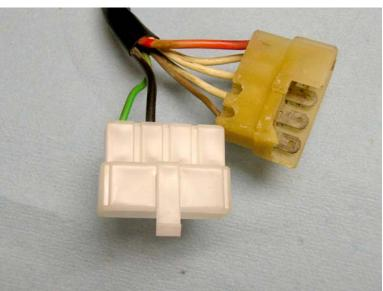
If you're moving wires over to a new shell like we're doing here, we suggest doing one at a time. This way, there's less chance of forgetting just exactly which wire goes where.
