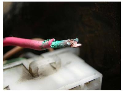
You're not the first, and you definitely won't be the last. Simple fix, right? Strip some insulation off the wire, crimp on a new connector, and you're back in business. (If it's corroded like this, you'll want to clean that up with baking soda/water, or if you have enough slack, cut off the corroded section of wire.)
