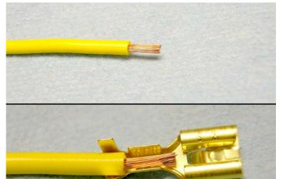
Here's how we go about it. For our example, we'll be using this 16 AWG size wire. First, grab your wire tool and strip off 5 or 6mm (1/4") of insulation – we don't want to take off more than that. Any more and you could find yourself unable to plug the male and female connectors all the way together because you have too much bare wire. Here you can see a good example of how it should look.
