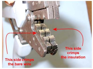
The neat thing about this setup is... instead of having to do two crimps (one for the wire and one for the insulation) we get to do both with one squeeze of the handle! The side with the AWG markings will actually be crimping the insulation, while the side with the metric markings will be crimping the bare wire. Ease and convenience in an easy to use package.
