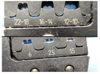
Here's a look at the dies that actually perform the crimp. One side has AWG (American Wire Gauge) markings, and the other metric. Yes, Virginia, there is more than one way to measure wire.
