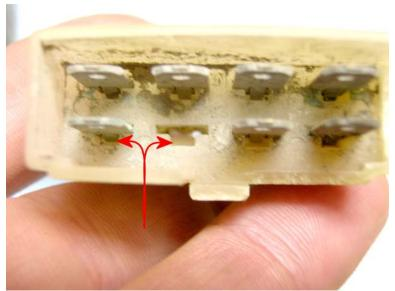
They're easy to use, too. Looking inside the shell, you'll notice the teensy slot below the terminal blade; that's where the retaining tab resides. Simply grab the appropriately-sized pick, push it into the slot, and if the wire is still attached, use it to gently pull the terminal out.
