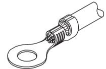
**Crimping Closed Barrel Terminals**
