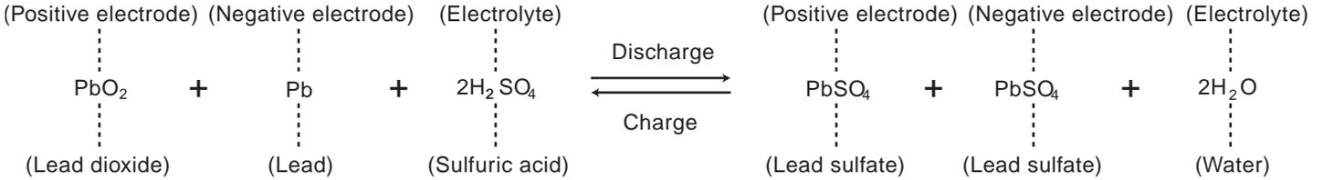
In the final stage of charging, an oxygen-generating reaction occurs at the positive plates. This oxygen transfers inside the battery, then is absorbed into the
