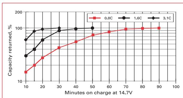
Table 7 shows that with a 0.8C<sub>10</sub> inrush current, a 100% discharged battery can have 80% of its capacity returned in 57 minutes; doubling the inrush to 1.6C<sub>10</sub> cuts the time taken to reach 80% capacity to only 28 minutes.
