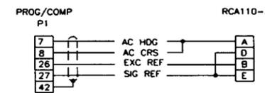
NOTE: SANDEL INDICATOR MUST BE CONFIGURED FOR KCS-55/5A HEADING SYSTEM.
