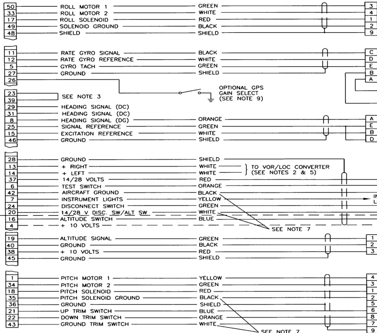
ADDITIONAL WIRING REQUIRED TO ADD PITCH SECTION (SYSTEM 50)
