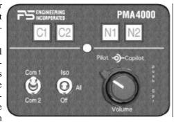
1) and "C2" (Com 2) push-buttons select the receiver, and are used to monitor a com that is not selected for transmit. You will <u>always</u> hear the audio from the transceiver that is selected by the 2-position mic selector toggle switch.
