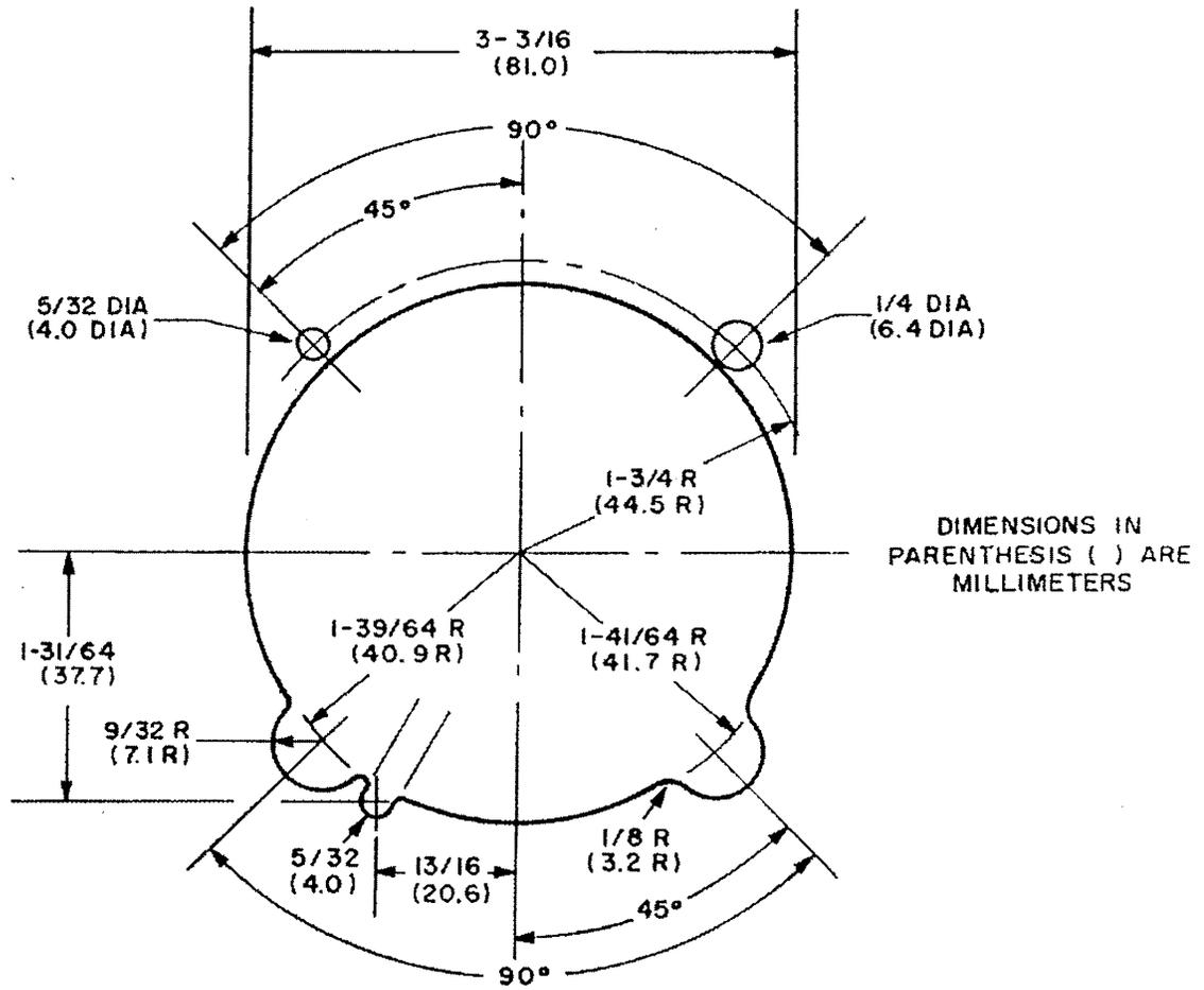
FIGURE 2-4. MOUNTING TEMPLATE, REAR MOUNT
