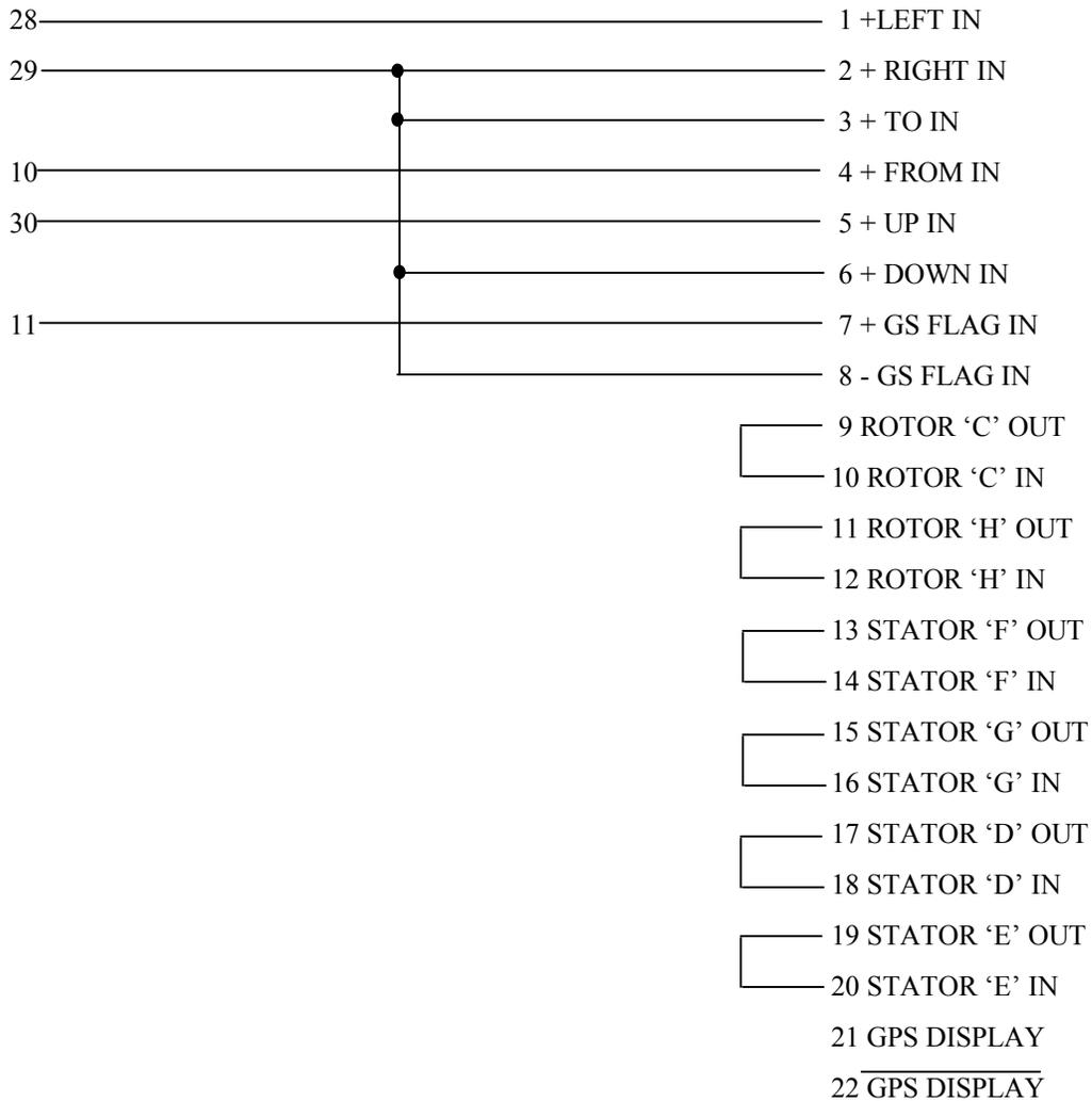
FIGURE 2-2 ADDITIONAL BENCH TEST HARNESS FOR NAV122D/GPS
