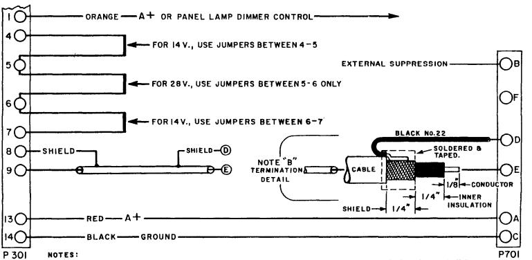
A - Do not ground the coax cable shield between the Panel Unit and the Remote Unit. The shield is grounded only at the Remote Unit end and any additional ground points will form ground loops which may cause false reply indications. The coax cable length is not critical, however, installations requiring a cable longer than 192", RG 58A/u should be used to minimize power loss.
