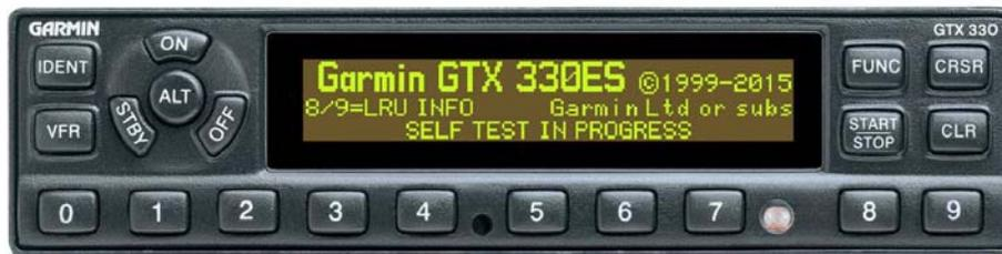
**Figure 1-2 GTX 330/330D Front Panel**
