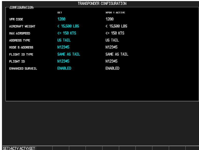
**Figure 6-38 GTX 335R XPDR Configuration**
