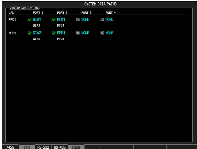
Figure 6-45 HSDB System Data Paths Unchecked GTS
