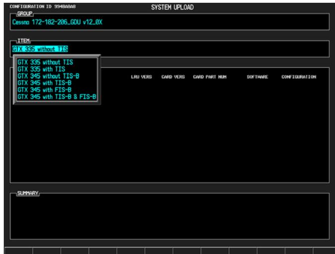
**Figure 6-34 GTX 335R System Upload Item**
