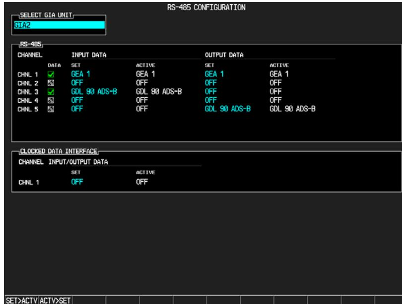
**Figure 6-59 GTX 345R GIA 2 RS-485 Configuration**
