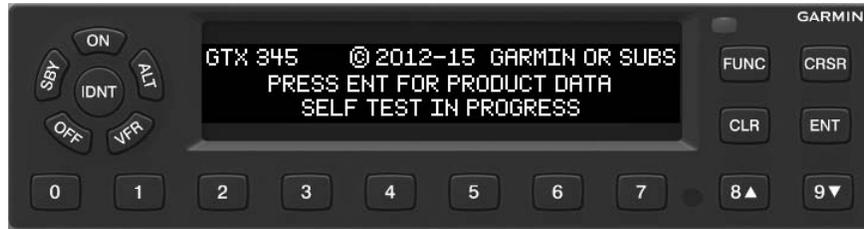
**Figure 5-3 GTX 3X5 Start-Up Screen**
