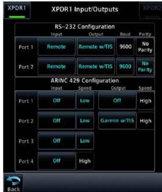
Figure 6-91 Inputs/Outputs Page
