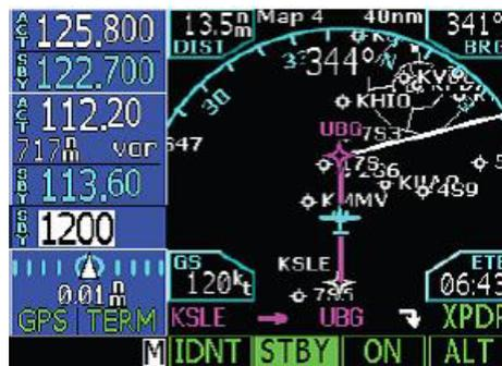
Figure 1-6 GNS 480 Transponder Control
