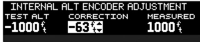
**Figure 6-15 Internal Alt Encoder Adjustment**
