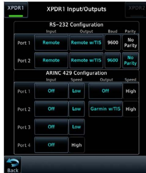
Figure 5-33. Remote XPDR Inputs/Outputs Page
