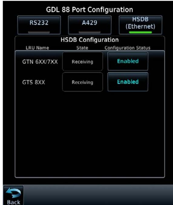
**Figure 5-46. GDL 88 Ethernet Configuration Page**
