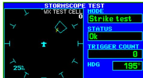
Figure 5-22. STORMSCOPE TEST Page
