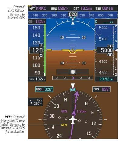
**External GPS Navigation Failure**
