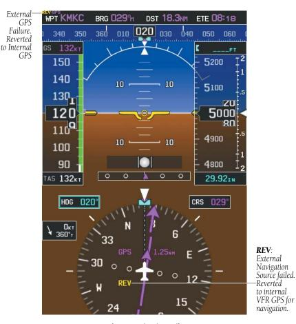
**External GPS Navigation Failure**
