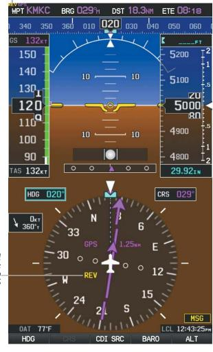
**REV**: External Navigation Source failed. Reverted tointernal VFR GPS for navigation.
