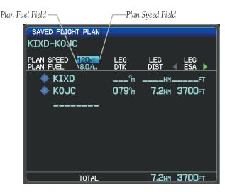
Plan Speed and Plan Fuel (Saved Flight Plan Page)
