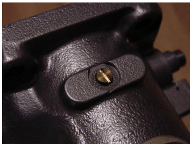
Figure 14-19 Carb Temp Sensor Mounting Location
