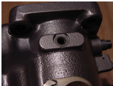
Figure 14-20 Carb Temp Sensor Mounting Location w/Screw Removed
