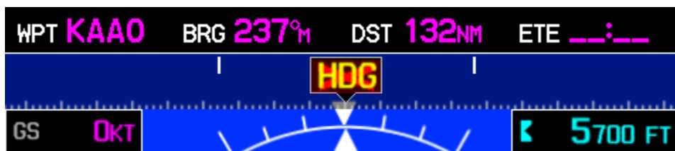
Figure 20-4 Heading Failure Indication (Full-Screen PFD)
