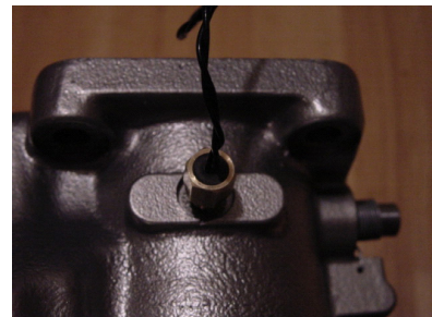
Figure 14-21 Carb Temp Sensor Installed
