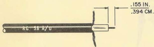
Separate braid into two equal parts and fold out to sides of coax. Shorten center conductor .100 inch and strip as shown.
