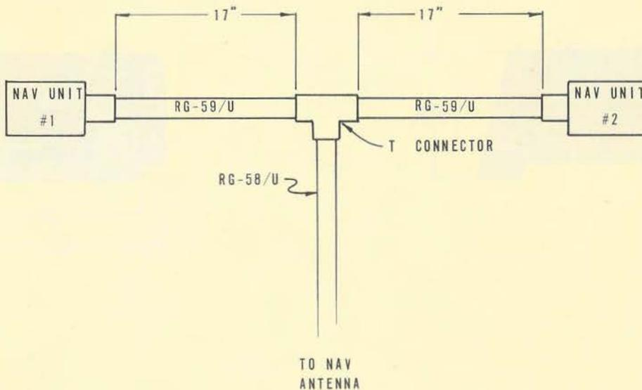
FIGURE 2-10 DUAL OMNI ANTENNA INSTALLATION
