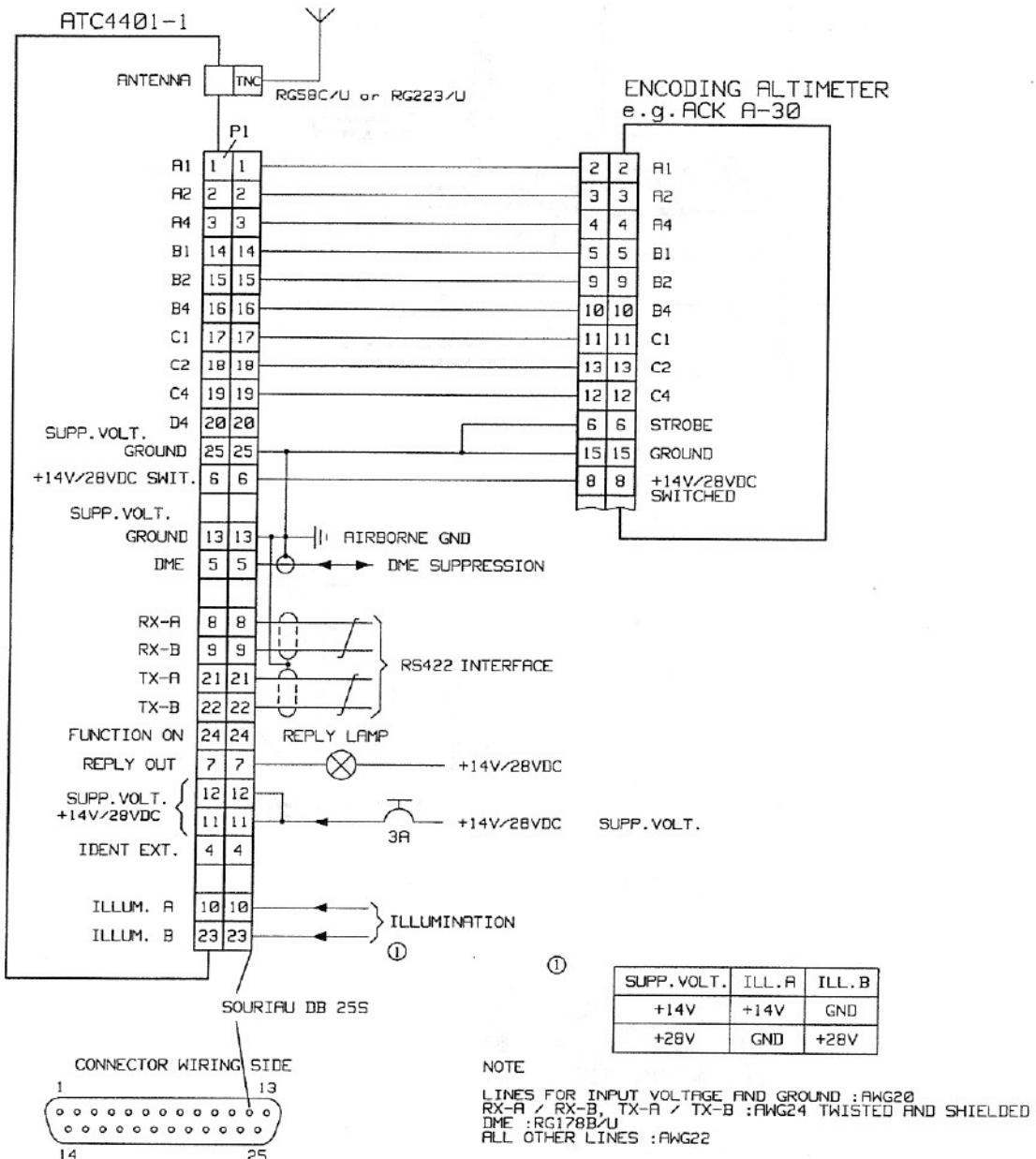
Fig. 2-4 Installation wiring ATC 4401-1 with encoding altimeter
